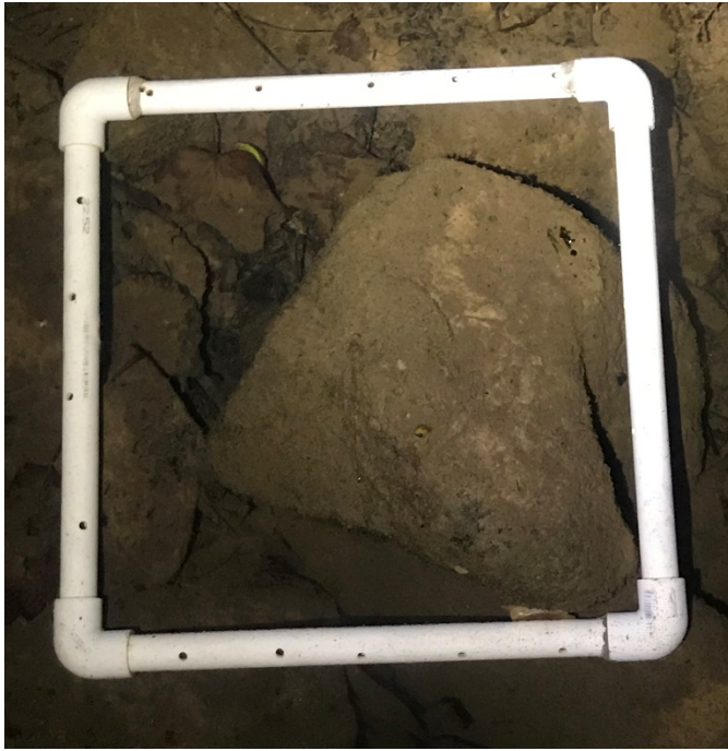
Figure 3. A 31x31 cm PVC square used as a sampling quadrat for collecting habitat data utilized to model habitat selection on multiple scales.
