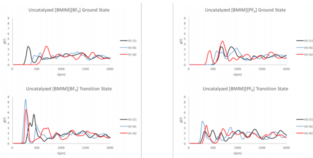
Figure 6.18. Radial distribution functions in [BMIM][BF 4 ] and [BMIM][PF 6 ] for the uncatalyzed MRH ground and transition states between H5 on BMIM and the oxadiazolic oxygen (H5-O1, black), oxadiazolic nitrogen (H5-N1, blue), and hydrazonic nitrogen (H5-N2, red)
