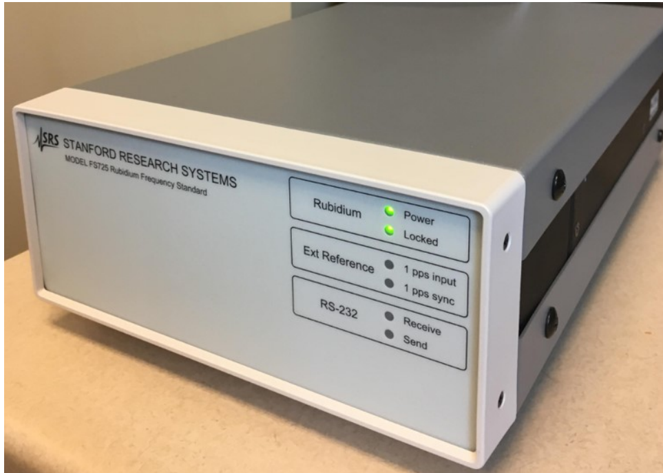
Figure C.8: Picture of the Rubidium Atomic Clock Tested in the Experiment
