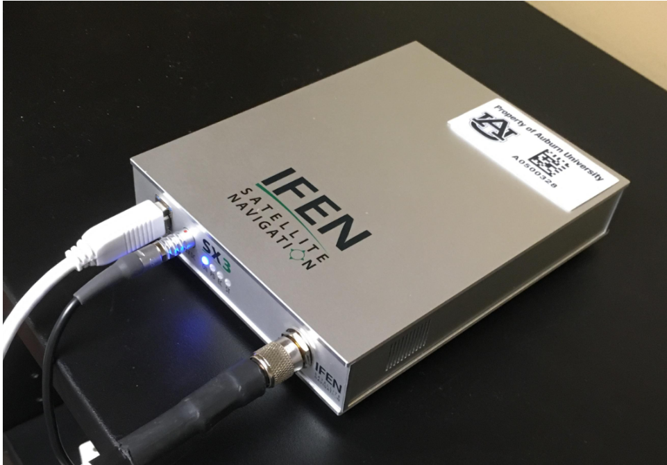
Figure 6.2: Picture of the IFEN SX3 Hardware Front-End
