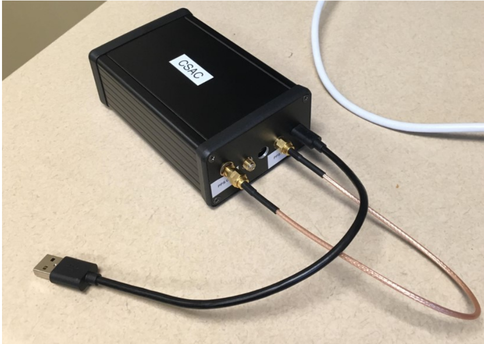
Figure C.12: Picture of the Cesium Atomic Clock Tested in the Experiment
