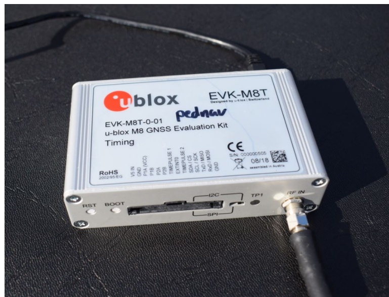
Figure 6.22: Picture of the GPS and GLONASS Ublox Receiver tested in the Experiments
