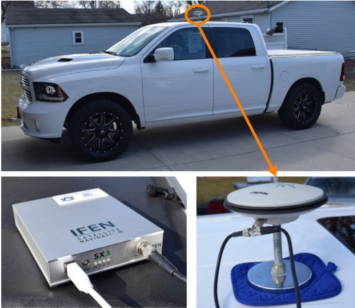
Figure 6.21: Setup of Signal Data Collection with Vehicle
