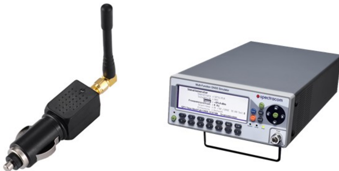
Figure 1.1: Jammer [7] and Simulator [17] Devices that can be used to degrade GPS
