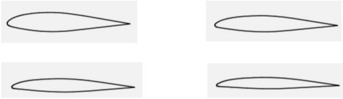
Figure 5.2: Boeing KC-135 Airfoils
