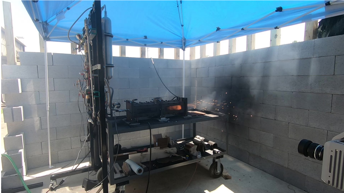
Figure 6.3: Hybrid rocket motor test fire using 0.05 inch diameter oxidizer injector and HDPE flow rate. The series of images shown in Figure 6.4 and Figure 6.5 show the combustion chamber when the popping noise was occurring. These images overlap the maximum pressure of the test. It can be seen that the combustion chamber goes dark in the first image then fires in the second then goes dark again in the third. The images in Figure 6.4 are taken from GoPro footage and the images in Figure 6.5 are taken from high speed video footage.
