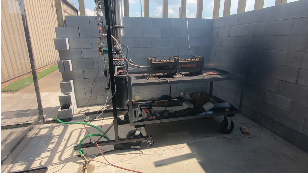
Figure 6.13: Hybrid rocket motor test fire using 0.08 inch diameter oxidizer injector and HDPE. Shows steady flame throughout the first 20 seconds of the test firing.
