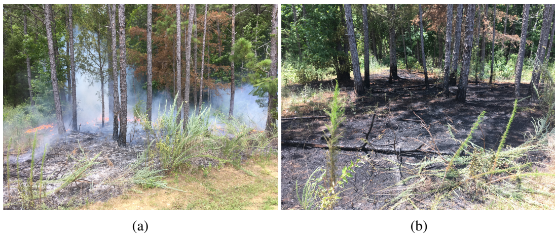
Figure 4.7: (a) During brush fire caused by ejected piece of igniter. (b) Post fire caused by ejected piece of igniter.
