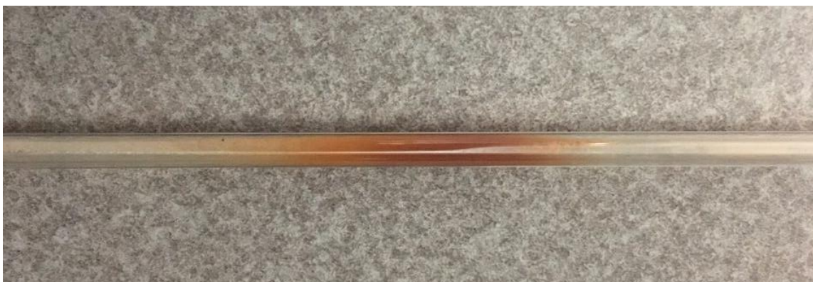
Figure 11. Capture of iron carbonyl by alumina powder.
