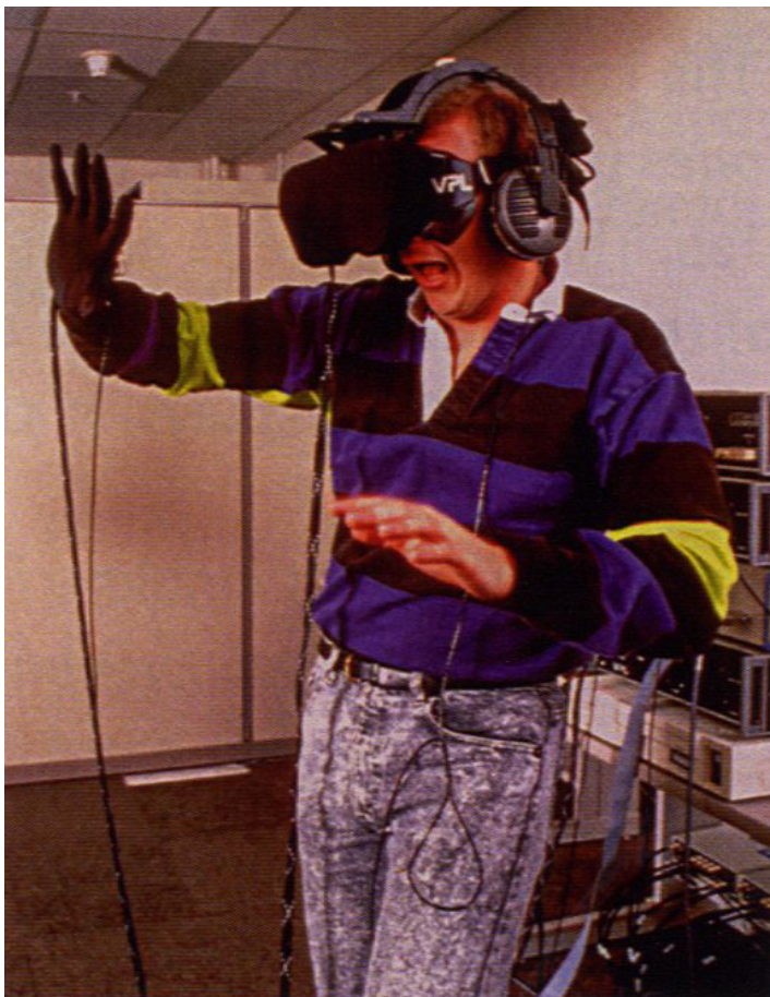
FIGURE 26 This user experiences and interacts with a virtual world using the VPL Eyephones and Datagloves. (Image courtesy of NCSA.)
