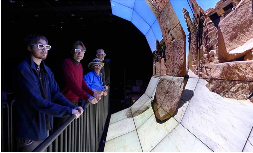
FIGURE 04 The Qualcomm Institute's WAVE provides the ability to look up and down in the virtual world by curving tiles around the horizontal axis. (Ramsey, 2015)
