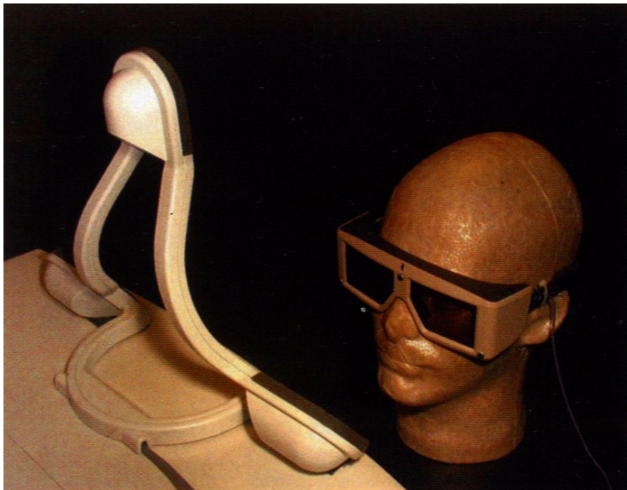
FIGURE 28 Logitech desktop 6-DOF tracking system based on ultrasonic signals which emanate from the three corners of the emitter and are transduced by microphones embedded in the active
