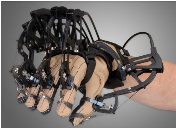
FIGURE 30 The CyberGrasp force feedback display (coupled with the CyberTouch input glove) uses a movement restriction technique to limit finger movement and thus provide feedback to the wearer's hand. (Image courtesy of CyberGlove systems Inc.)
