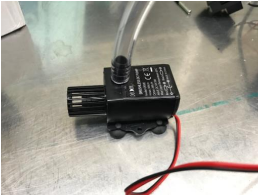
Water pump (Decdeal Submersible Water Pump DC 12V 5W Model: QR50E)
