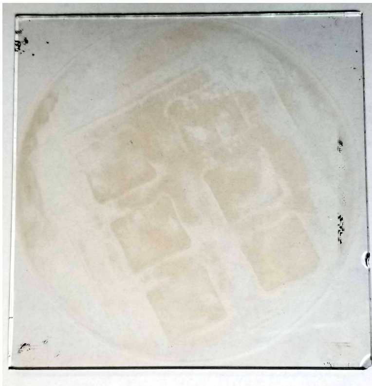
Figure 6-1 Results of plasma etching on glass square in the presence of the "waffle" electrode. The piece of glass was used to cover the hole in the top rf electrode within the MDPX vacuum chamber.
