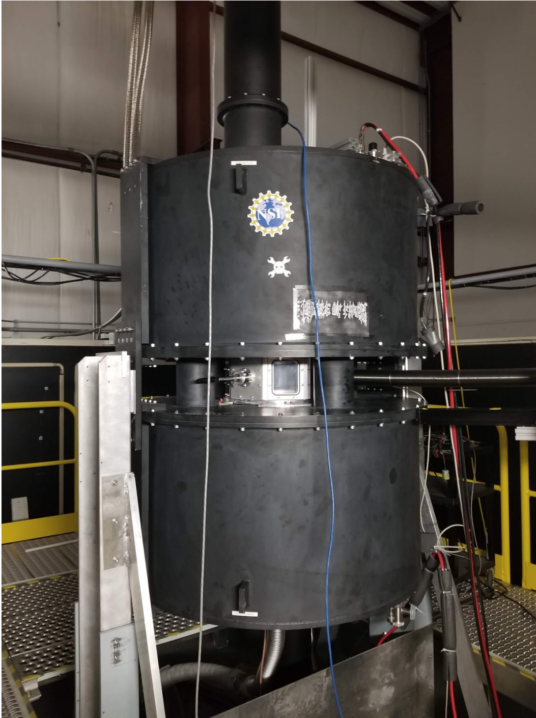
Figure 2-1 The Magnetized Dusty Plasma Experiment (MDPX). Two magnet coils reside in each of the black cylinders. Cryostats above and below the magnet (just out of frame) pull heat out of the coil cooling them to 4-5 K. The octagonal vacuum vessel can also be seen in the center. This split-bore design allows for greater optical and diagnostic access to experiments. [38,39]
