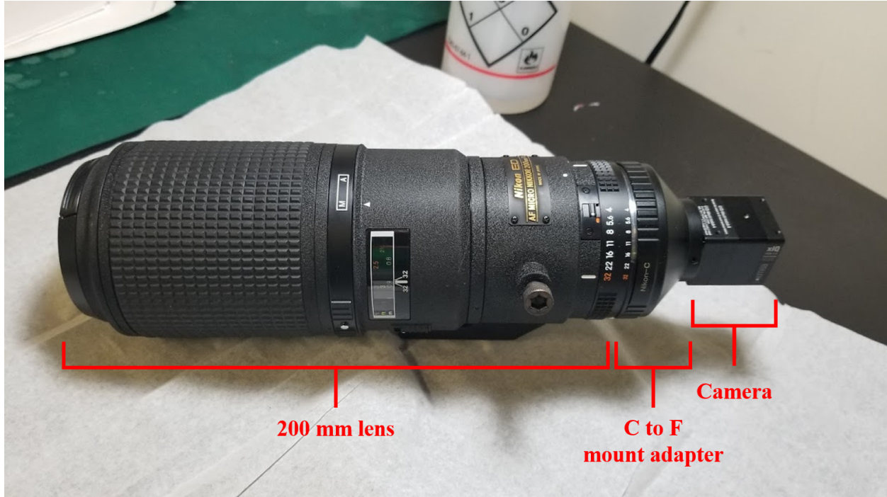
Figure 2-6 Image of Nikon 200 mm lens and Ximea camera.
