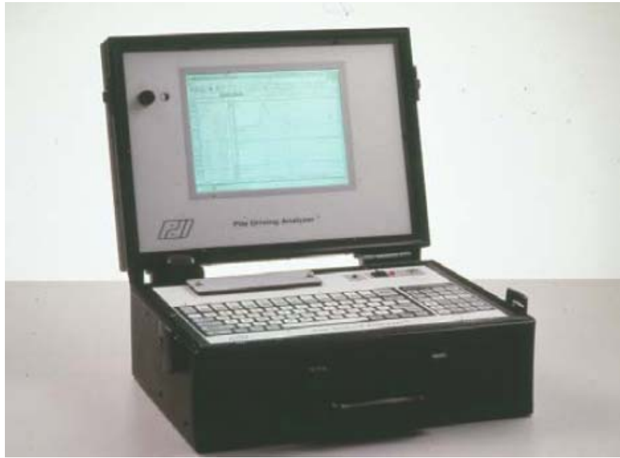
Figure 1-2. Pile Driving Analyzer (FHWA, 1997)
