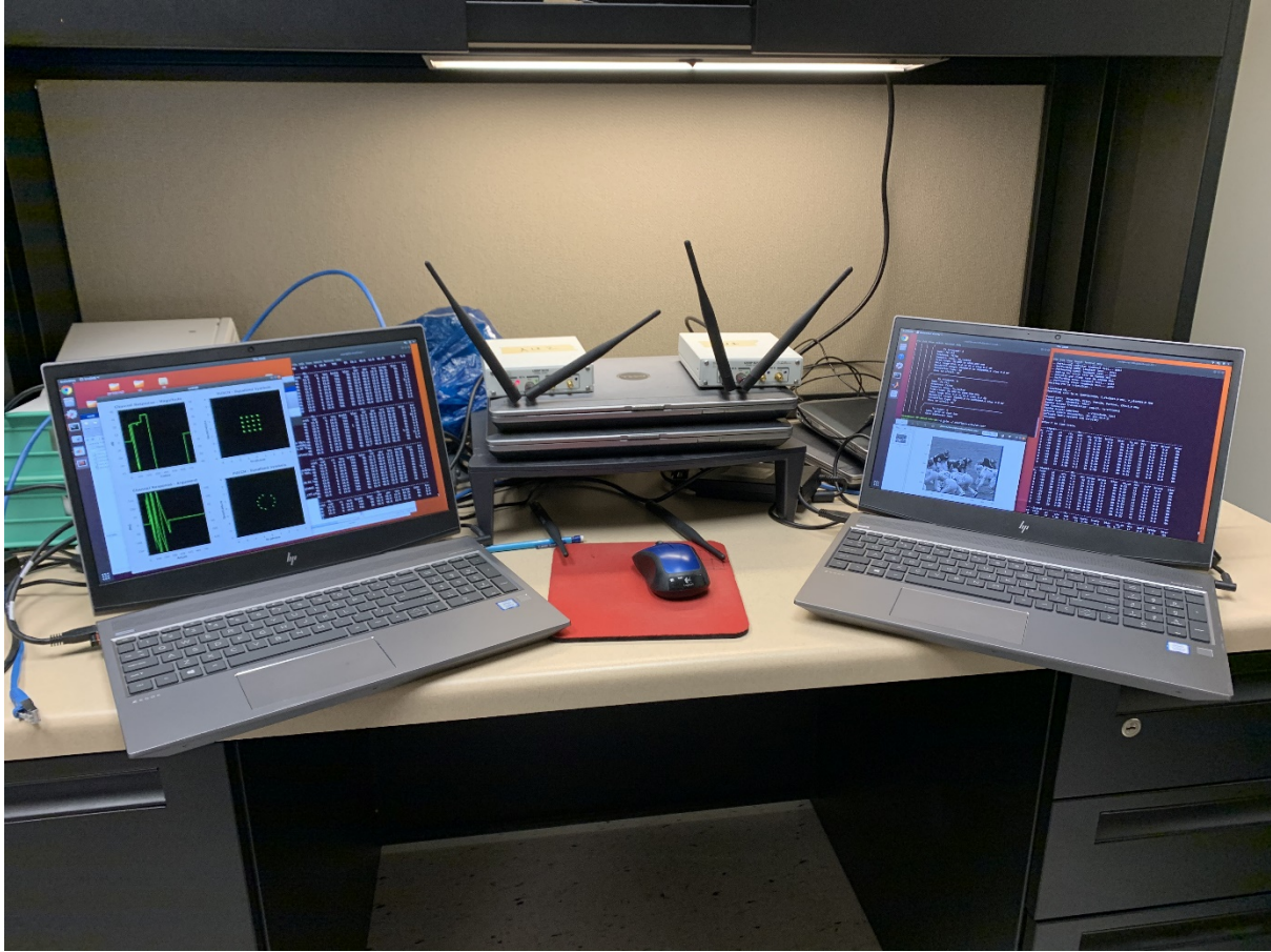
Figure 5.1: The configuration of the sender (left) as the eNB and the receiver (right) as the UE.
