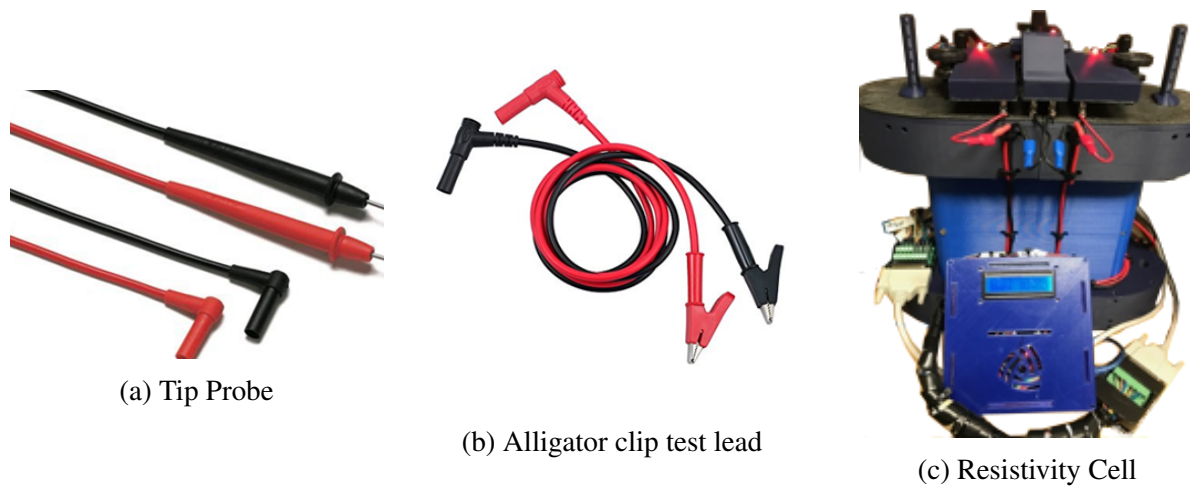
Figure 2.5: Electrodes and Fixture used in metrology systems
