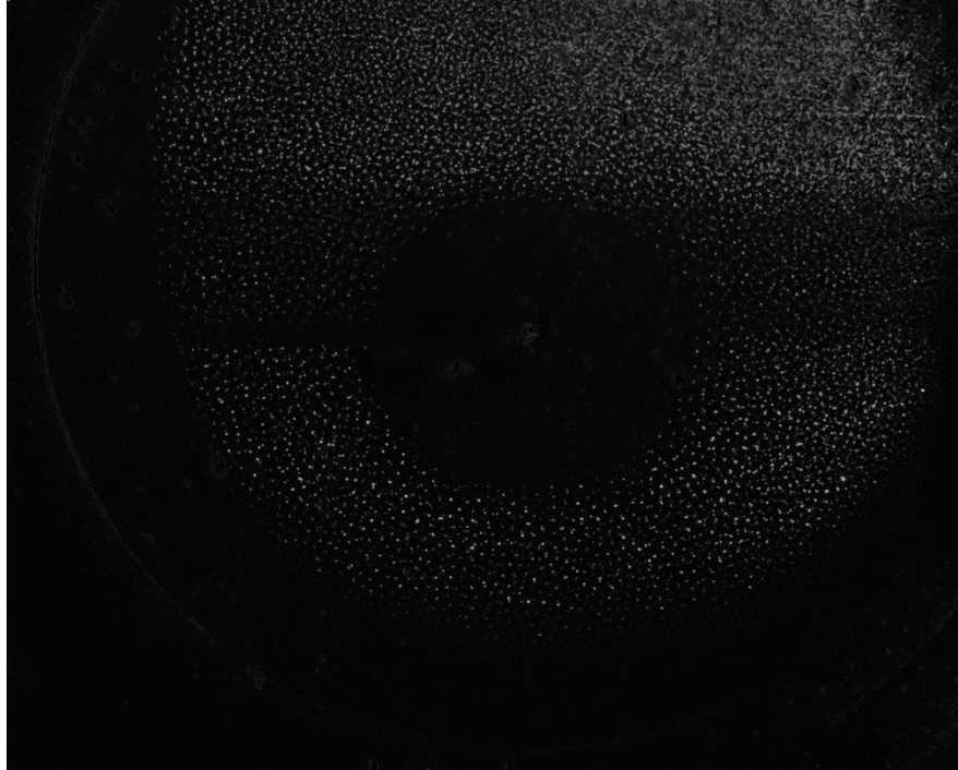
Figure 4-3: A single frame (out of 300) of a background-removed video. Other than a few very minimal artifacts (for instance, slight reflections from the base of the probe and the confining ring), only the floating dust grains remain. The shadow of the probe tip in the laser light sheet can be seen to the left of the dust ring (at the approximately 9:00 position). The structure of the dust void is now much more plainly visible to the naked eye. Additionally, the dust particles that were originally obscured by the background in the upper half of the original image can now be clearly identified in this image.
