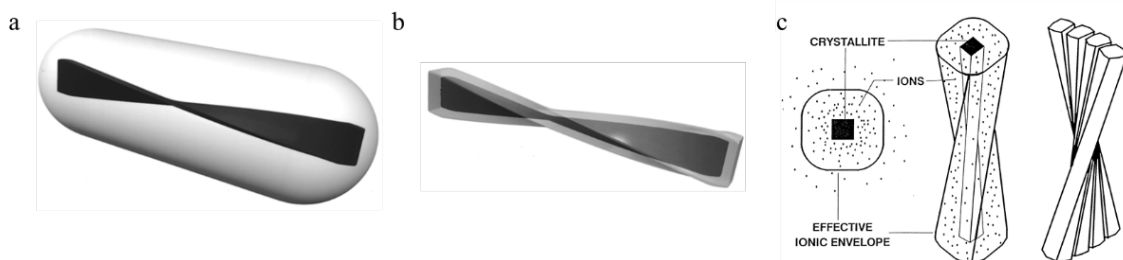
Figure 2.24: An illustration of the twisted structure of CNC with surrounding effective ionic envelope a) before and b) after NaCl addition, and c) labeled schematic of the effective ionic envelope and the ordering behavior of a twisted rigid rod. 102-103
