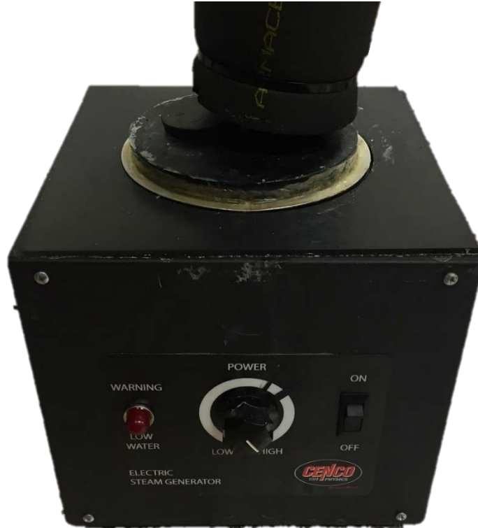
Figure 4: Photo of steam generator
