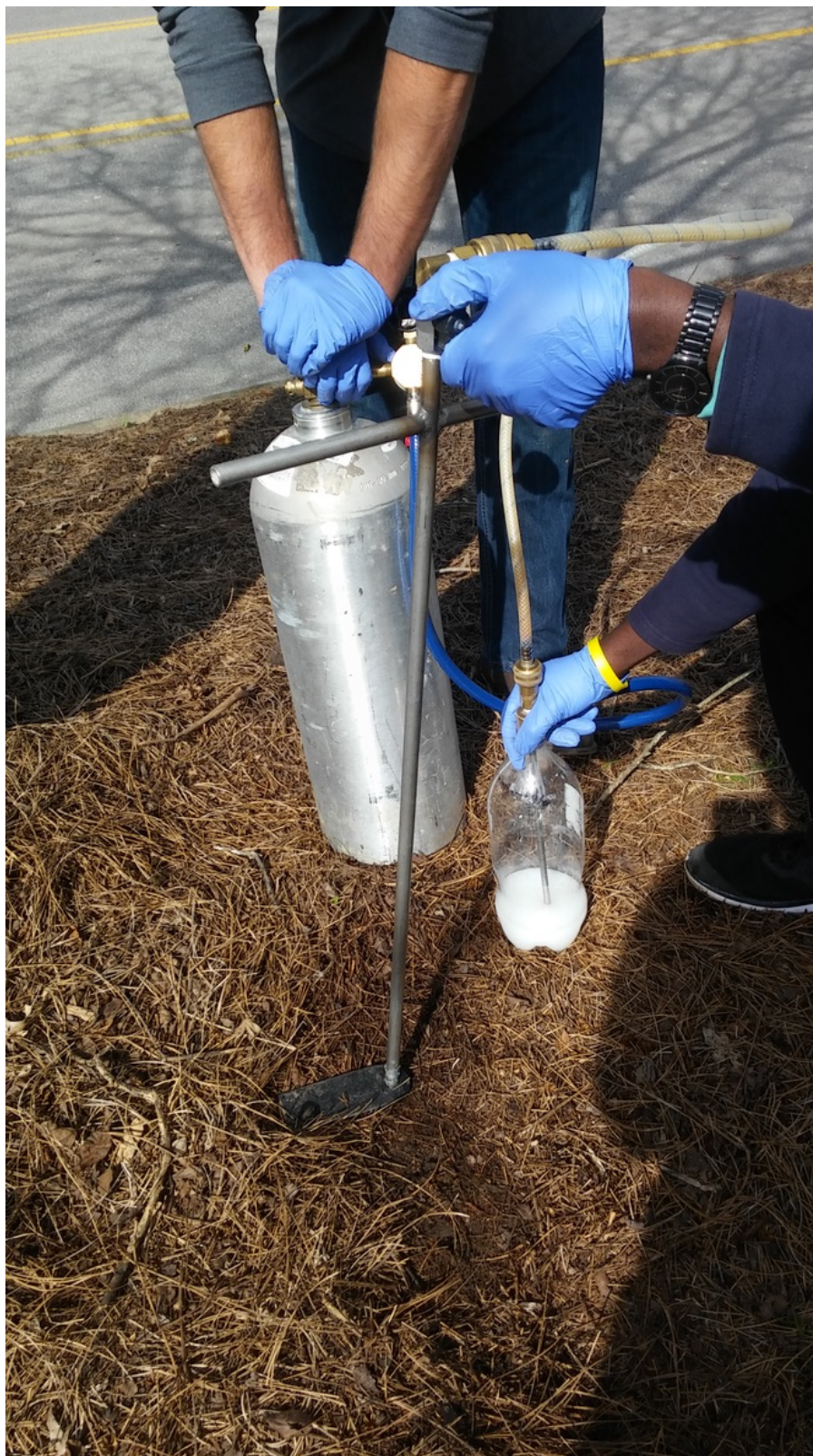
Figure 11. CO 2 tank and soil injector rod.
