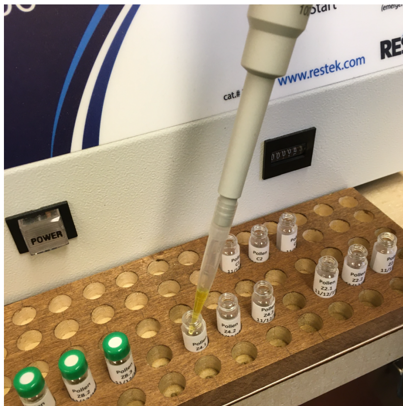
Figure 30. Transfer of supernatant to glass LC-MS vials for storage prior to injecting.
