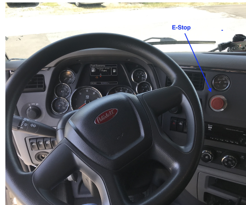
(b) Emergency switch placement
