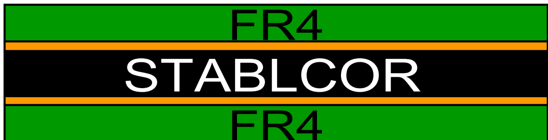
Figure 8.1 - Example Hybrid PCB Laminate Incorporating Low CTE Carbon Fiber Based Core (STABLCOR)
