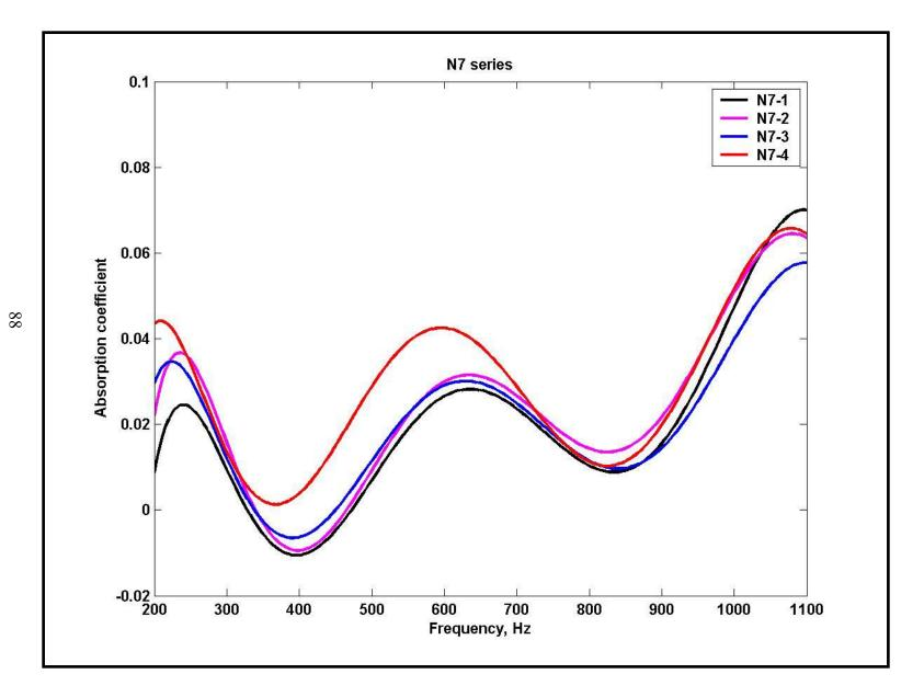
Figure 6.9 Absorption coefficient of sample N7 using 6-inch tube
