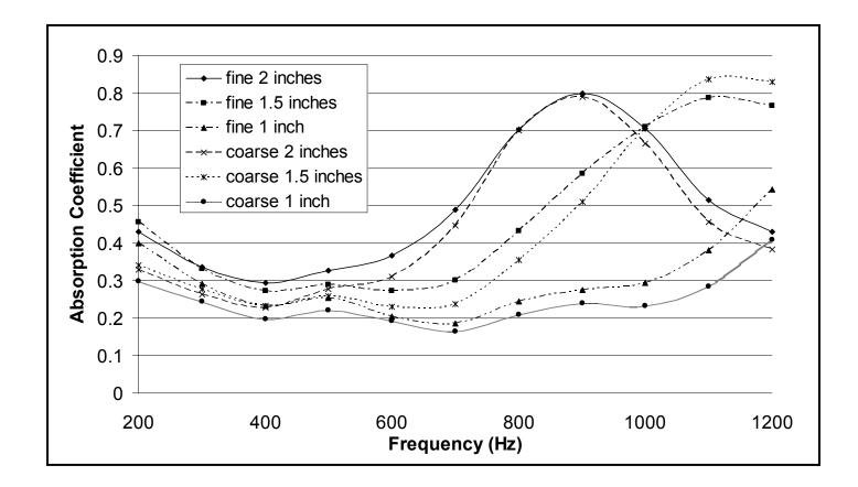
Figure 6.25 Comparison of sound absorption coefficients of OGFC slabs measured by the 6-inch tube
