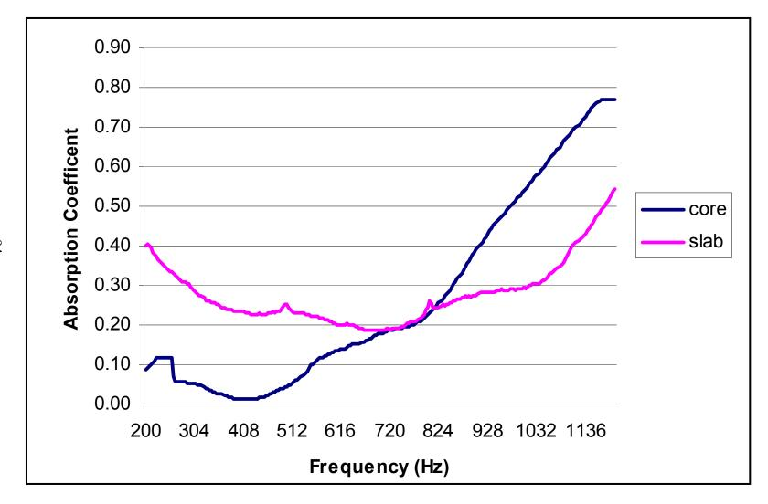
Figure 6.15 Sound absorption coefficients of OGFC 1.5-inch fine cores measured by a 6-inch tube
