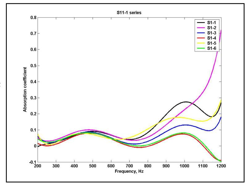
Figure 6.7 Absorption coefficient of sample S1 using 6-inch tube
