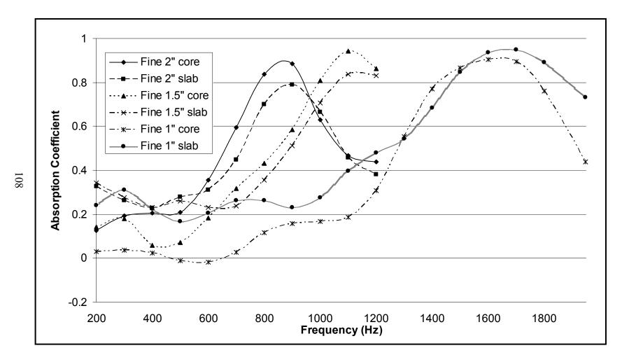
Figure 6.29. Comparison of the sound absorption coefficient of OGFC aggregated fine slabs and cores
