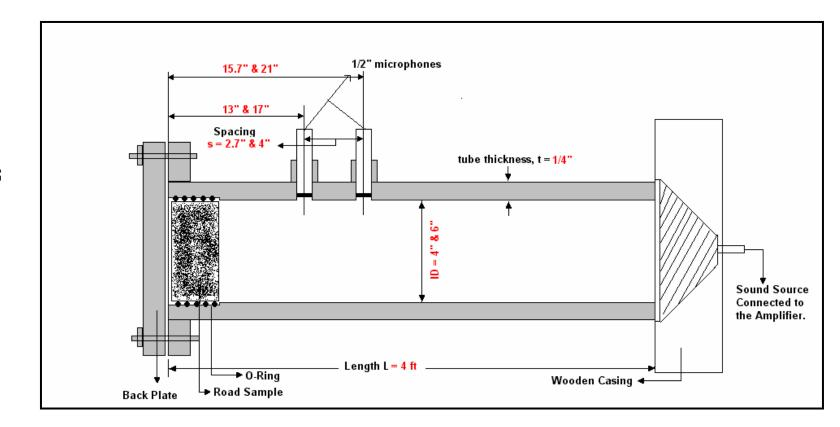
Figure 4.3 Dimensions of the two-microphone impedance tube built at Auburn University
