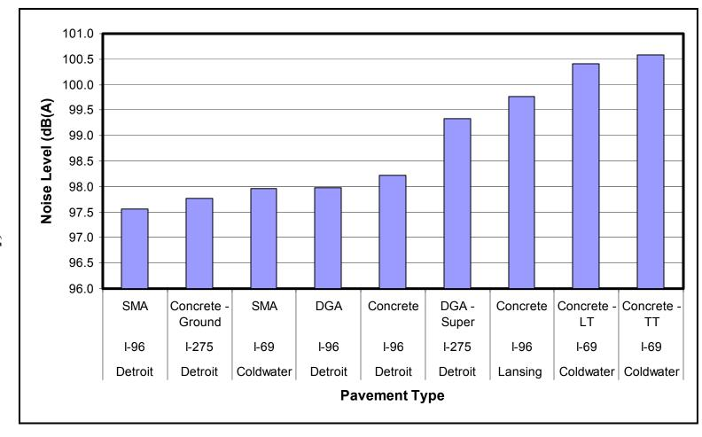
Figure 5.1.5 – Comparison of noise levels for different surfaces
