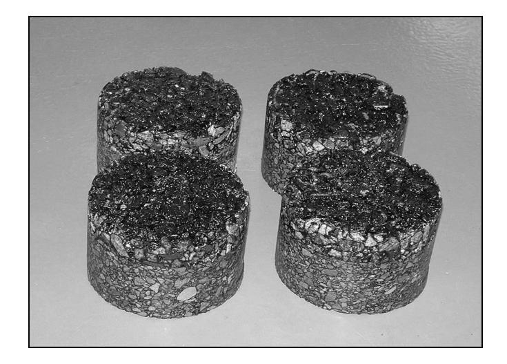
Figure 6.13. OGFC graded coarse 1.5-inch thick 6-inch diameter porous cores
