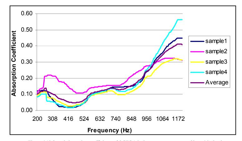
Figure 6.19 Sound absorption coefficients of OGFC 1-inch coarse cores measured by a 6-inch tube
