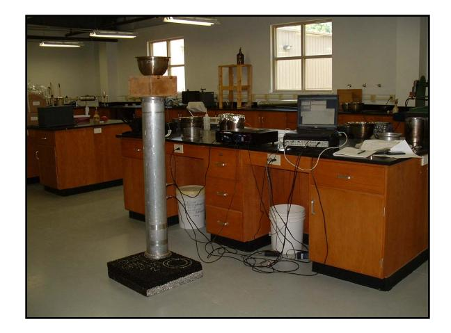
Figure 6.26. Experimental setup for in situ measurements of sound absorption coefficient of slabs
