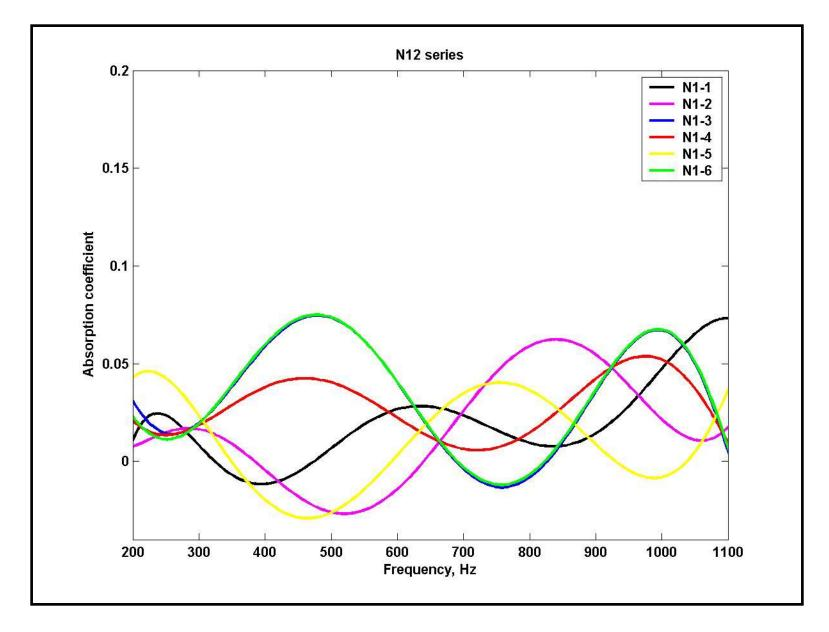
Figure 6.10 Absorption coefficient of sample N1 using 6-inch tube
