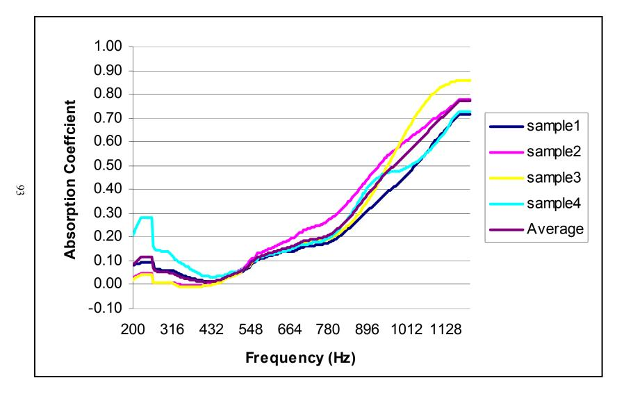
Figure 6.14 Sound absorption coefficients of OGFC 1-inch fine cores measured by a 6-inch tube
