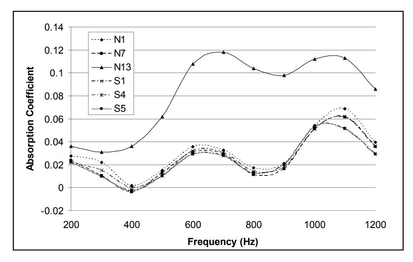
Figure 6.12. Comparison of the sound absorption coefficients of hard samples measured in the 6-inch tube
