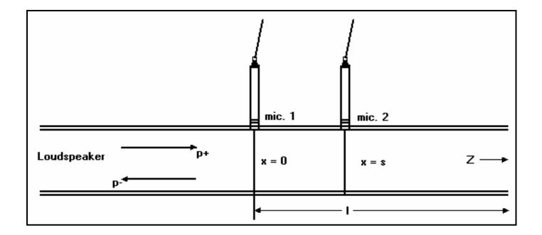
Figure 4.2 Impedance tube set up
