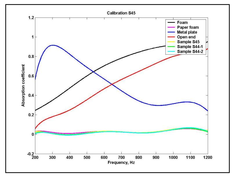
Figure 6.4 Comparison of sound absorption coefficients of different samples using 6-inch tube
