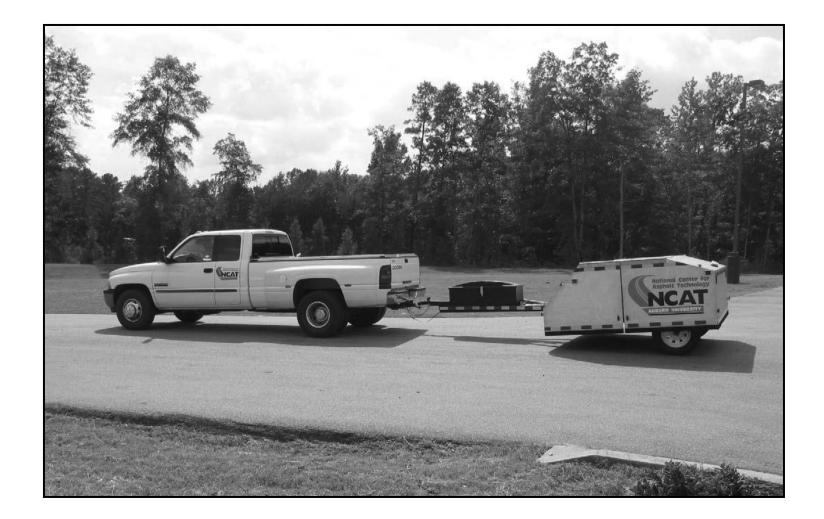
Figure 6.31. NCAT tire noise measurement trailer set-up
