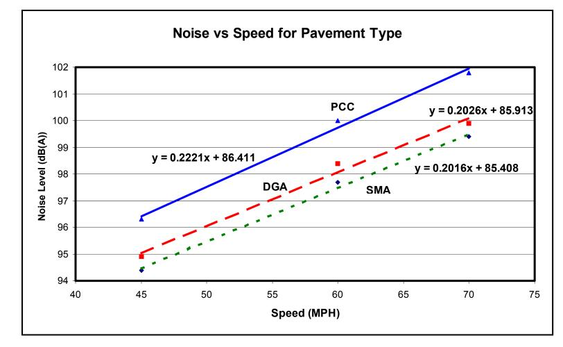
Figure 5.1.7 – Noise versus speed
