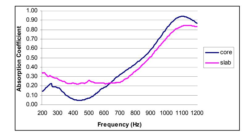
Figure 6.22 Comparison of sound absorption coefficients of OGFC coarse 1.5-inch core and slab measured by 6-inch tube
