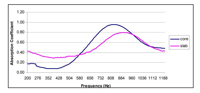
Figure 6.18 Comparison of sound absorption coefficients of OGFC fine 2-inch core and slab measured by 6-inch tube
