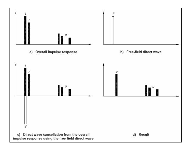
Figure 5.2.3 Principle of the signal subtraction technique I = direct incident wave, r = reflected wave, u = unwanted parasitic
