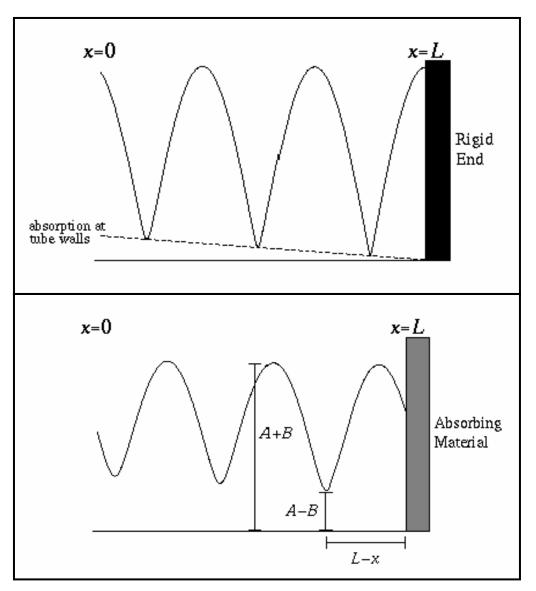
Figure 4.1 a and b Standing wave pattern in the impedance tube
