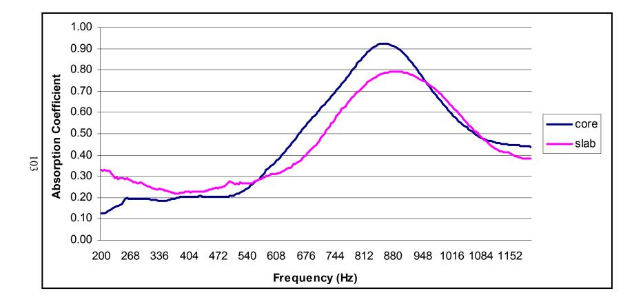
Figure 6.24 Comparison of sound absorption coefficients of OGFC coarse 2-inch core and slab measured by 6-inch tube
