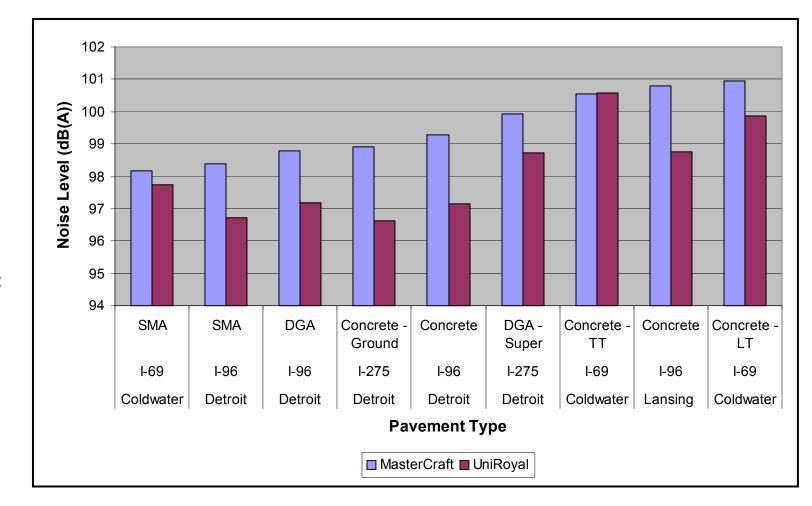
Figure 5.1.6 – Comparison of noise levels for each of the tires
