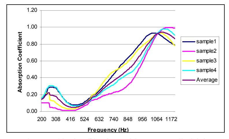
Figure 6.21 Sound absorption coefficients of OGFC 1.5-inch coarse cores measured by 6-inch tube
