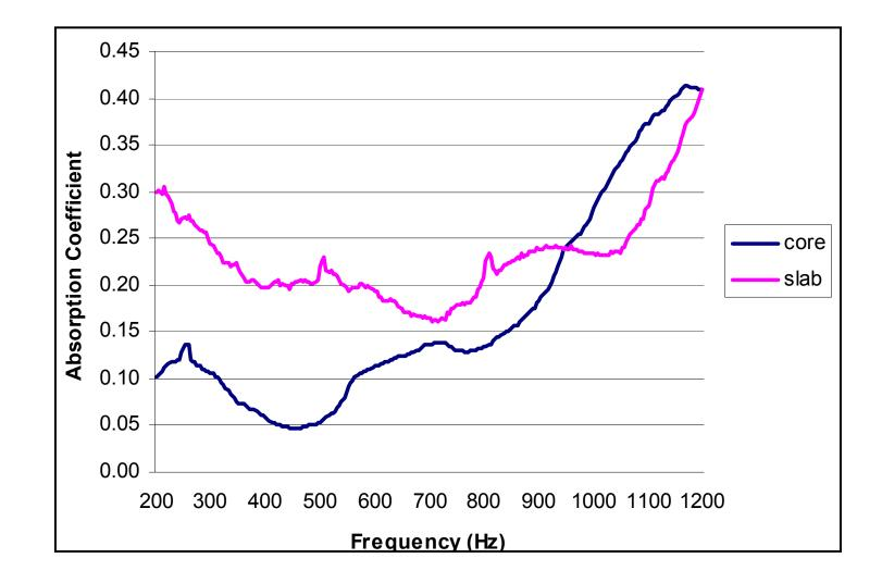
Figure 6.20 Comparison of sound absorption coefficients of OGFC coarse 1-inch core and slab measured by 6-inch tube
