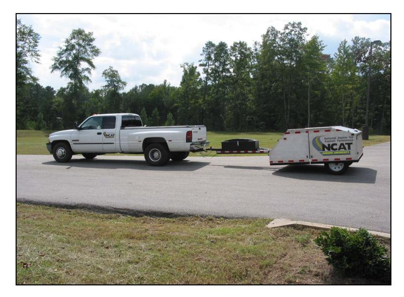
Figure 5.1.2 – NCAT CPX trailer
