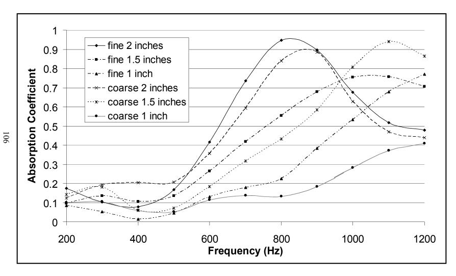
Figure 6.27. Comparison of sound absorption coefficients of OGFC cores measured in 6-inch tube
