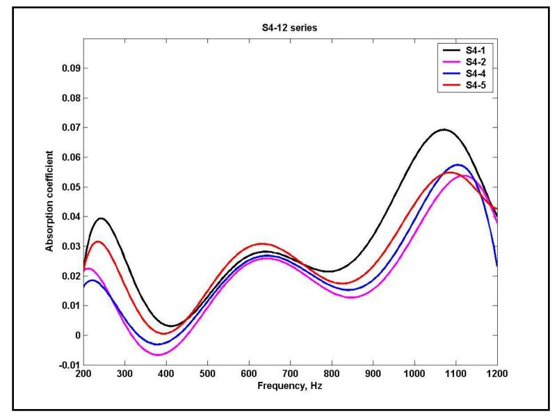
Figure 6.5 Absorption coefficient of sample S4 using a 6-inch tube
