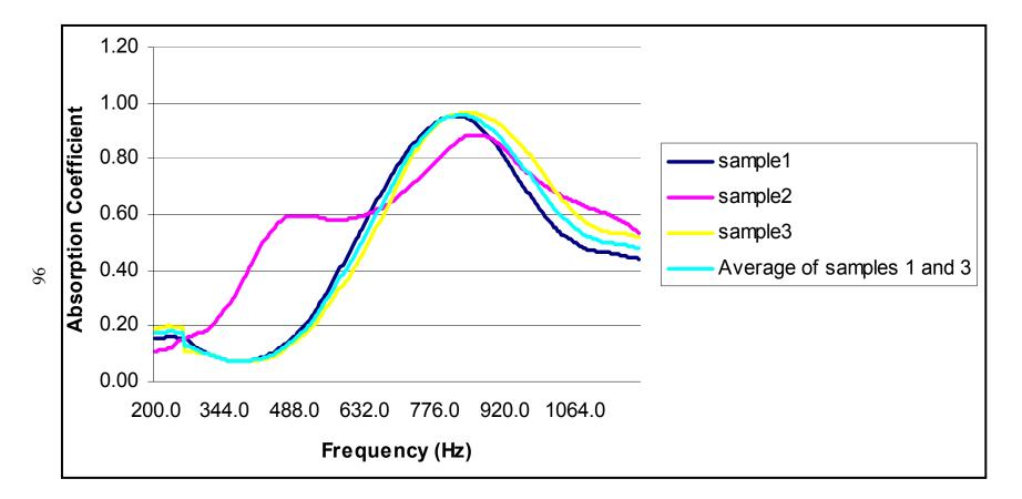
Figure 6.17 Sound absorption coefficients of OGFC 2-inch fine cores measured by a 6-inch tube
