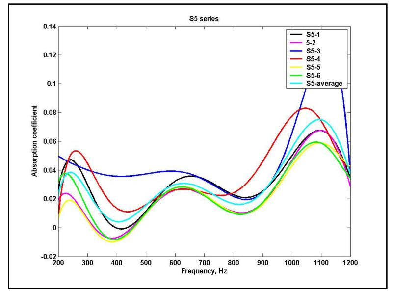
Figure 6.6 Absorption coefficient of sample S5 using 6-inch tube
