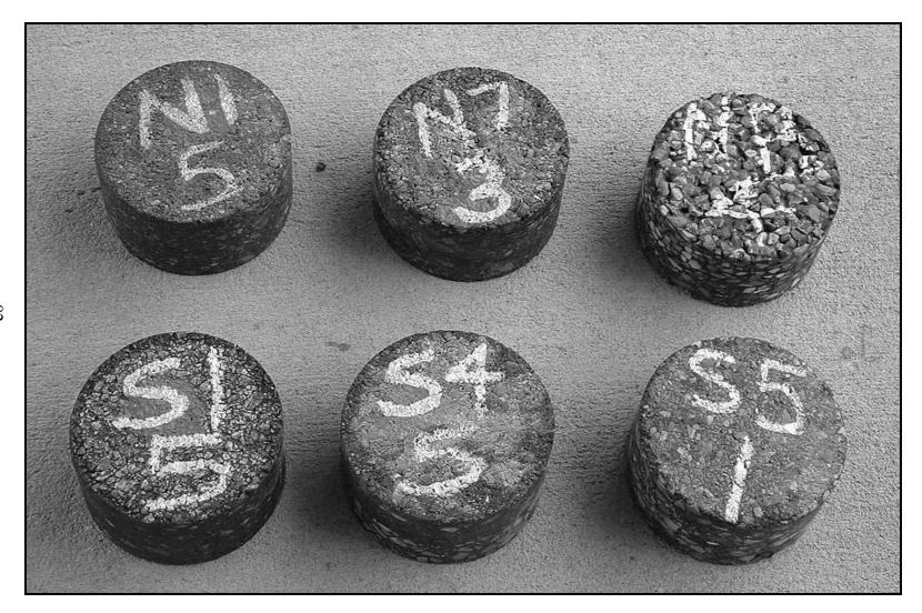
Figure 6.3. The 3-inch thick hard surface dense track pavement samples
