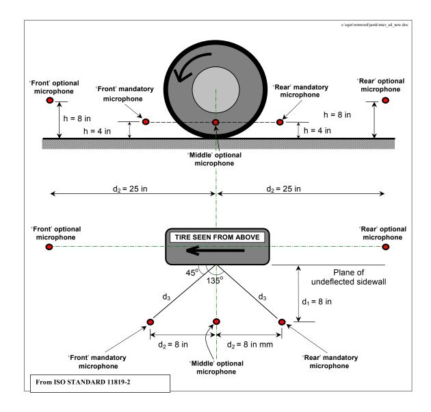
Figure 5.1.1. Microphone layout for close-proximity method (trailer method)
