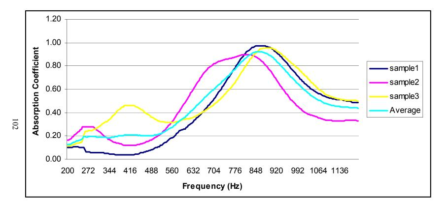
Figure 6.23 Sound absorption coefficients of OGFC 2-inch coarse cores measured by a 6-inch tube
