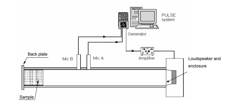
Figure 6.1. Experimental setup of impedance tube
