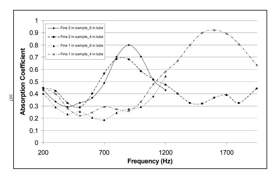
Figure 6.28. Comparison of sound absorption coefficients of OGFC slabs measured by 6-inch and 4-inch tubes
