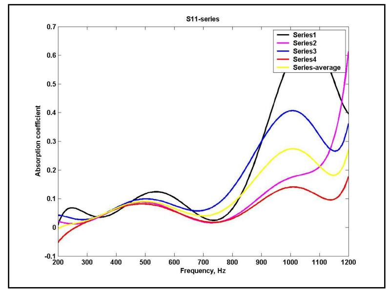
Figure 6.8 Absorption coefficient of sample S11 using 6-inch tube
