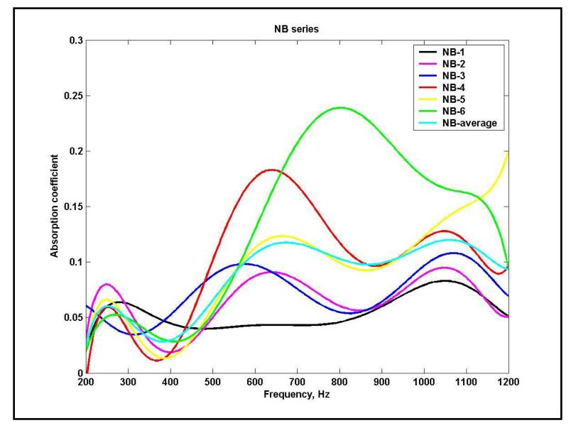
Figure 6.11 Absorption coefficient of sample NB using 6-inch tube
