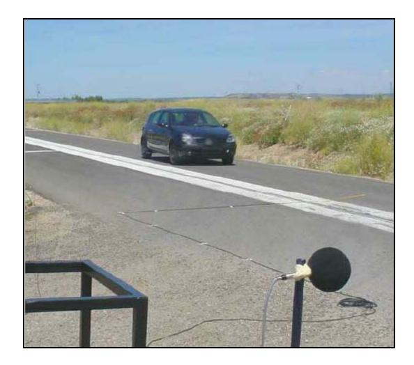
Figure 5.3.1. Measurement Set-up for statistical pass-by method
