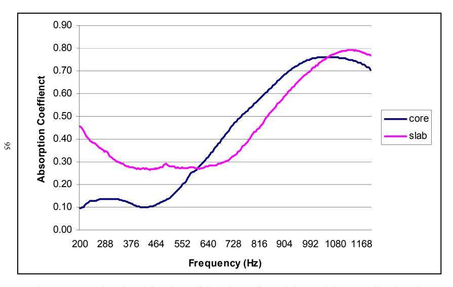
Figure 6.16: Comparison of sound absorption coefficients of OGFC fine 1.5-inch core and slab measured by 6-inch tube
