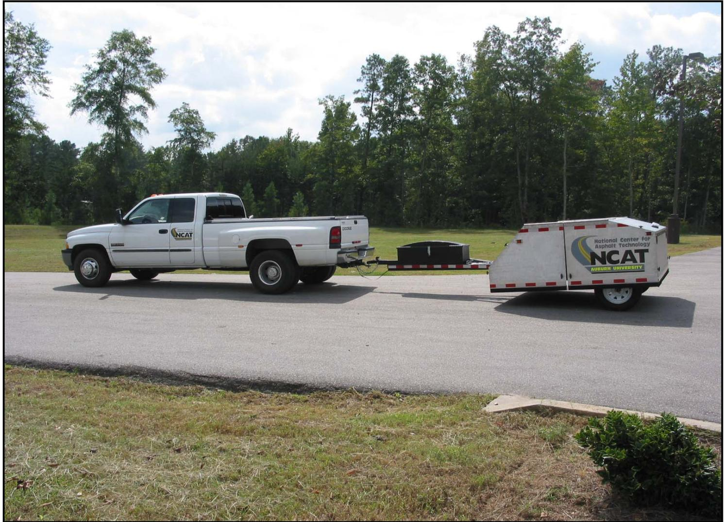
Figure 5.1.2 – NCAT CPX trailer
