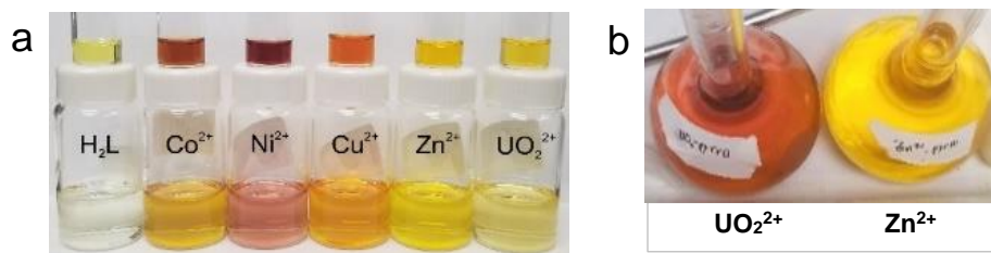
Figure 4.12 (a) 500 \mu\text{M} (upper vials) and 50 \mu\text{M} (lower vials) colorimetric series of \text{H}_2\text{L}^1 and complexes in 9:1 THF:MeOH (v/v); (b) top-down views of \text{UO}_2\text{L}^1 (right) and \text{Zn}_2(\text{L}^1)_2 (left) solutions, 500 \mu\text{M} in \text{CH}_3\text{CN} .
