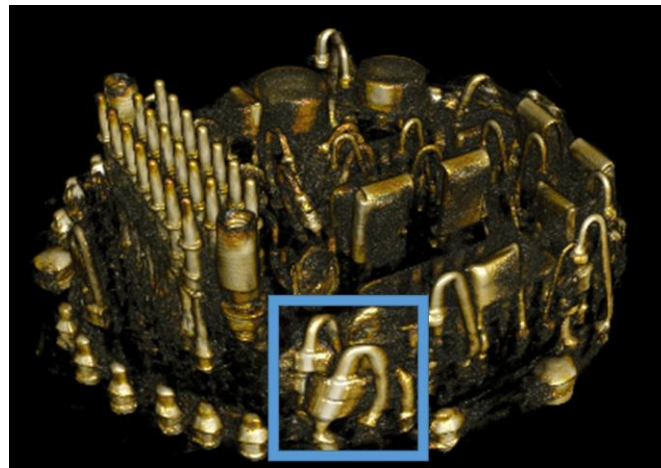
Figure 81: Location of the electrical component on the top board assembly
