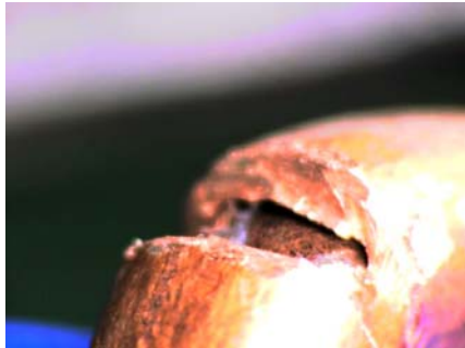
(a) No damage to wick due to bending (90°) (10x magnification)
