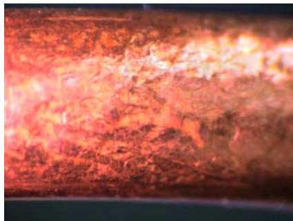
(e) Bended heat pipe outer wall (5x magnification)
