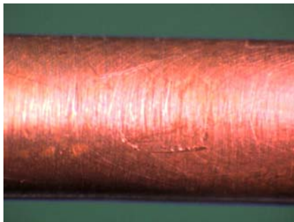
(c) Straight heat pipe wall texture (5x magnification)
