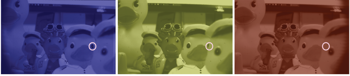
Figure 3.8: Multi-band perspective shift of rubber ducks at different depths. The white circle is placed at the same location on the images to show the movement of the ducks.
