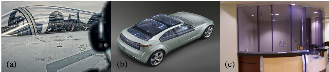
Figure 1-1: Examples of transparent composite applications (Sources: (a) www.defencetalk.com , (b) www.cbsistatic.com , (c) www.bulletresistant.bulletguard.com )
