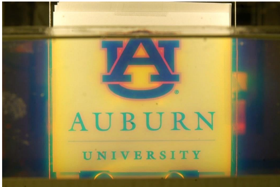
Figure 2-9: Optical transparency of fully cured glass-filled epoxy material (10% volume fraction, Time = 9 hours)
