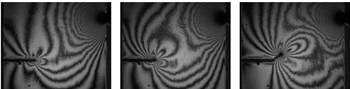
Figure 6-5: Isochromatic fringe patterns for 0%, 5%, 10%, and 15% V_f composites under dynamic mixed-mode loading ( a/W = 0.3 ). Images are shown for t = -20 \mu s , 0 \mu s , and 20 \mu s shown ( t = 0 corresponding to crack initiation)
