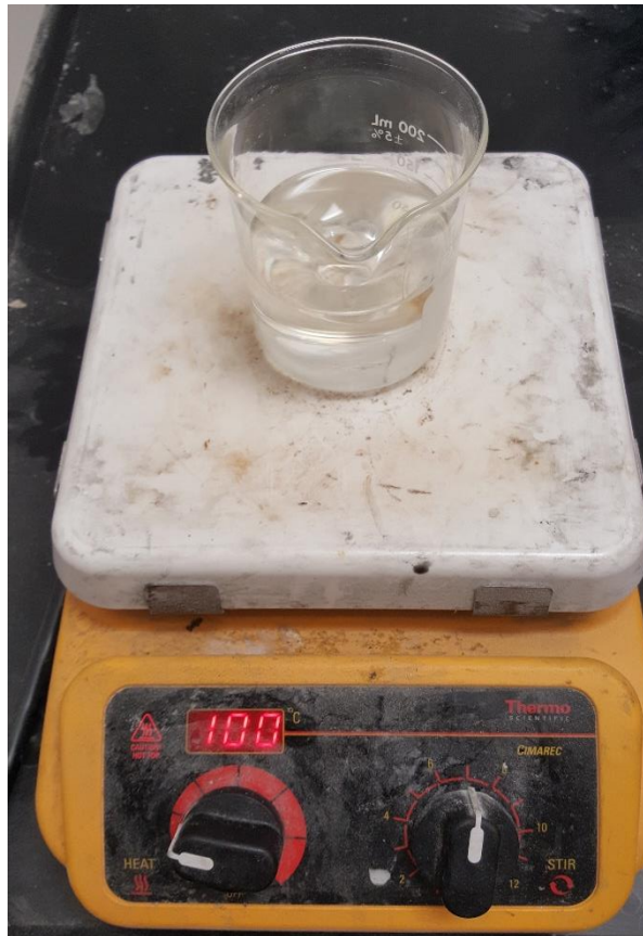
Figure 2-3: Photograph Epoxy resin and glass fiber mixture in 300mL beaker placed on a hot plate during magnetic stir bar mixing
