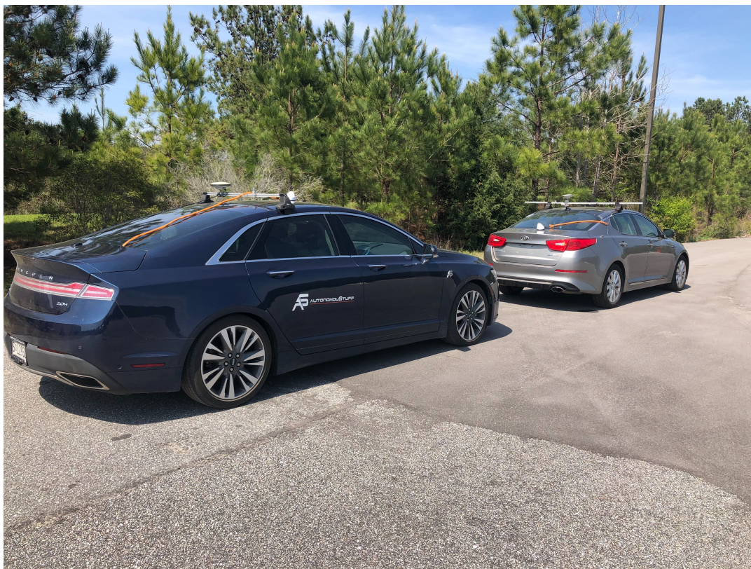
Figure 5.49: MKZ Test Vehicle Setup as an Autonomous Follower to the Manually Driven Kia Optima Leader Vehicle
