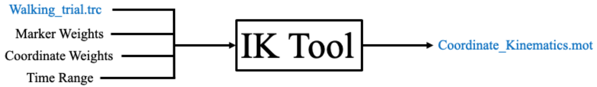
Figure 31: Inputs and outputs for the Inverse Kinematics Tool in OpenSim. Imported files are blue while user defined inputs are black
