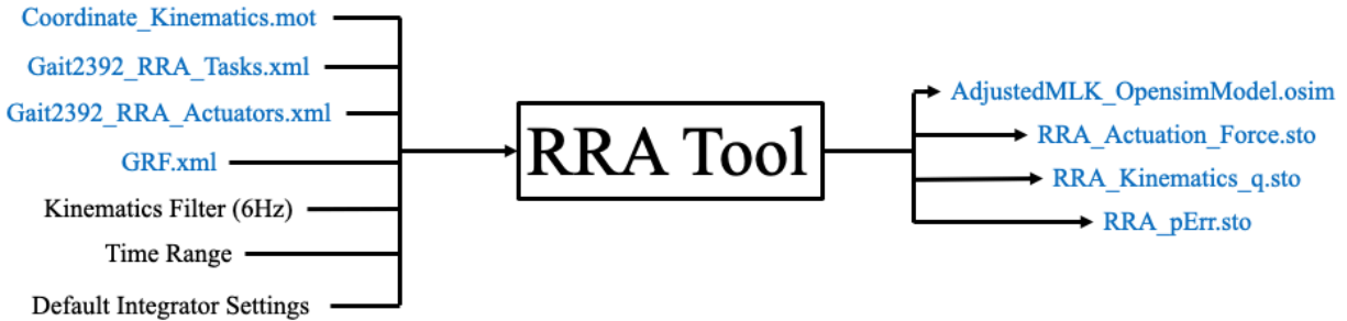
Figure 32: Inputs and outputs for the Residual Reduction Analysis (RRA) Tool in OpenSim. Imported files are blue while user defined inputs are black
