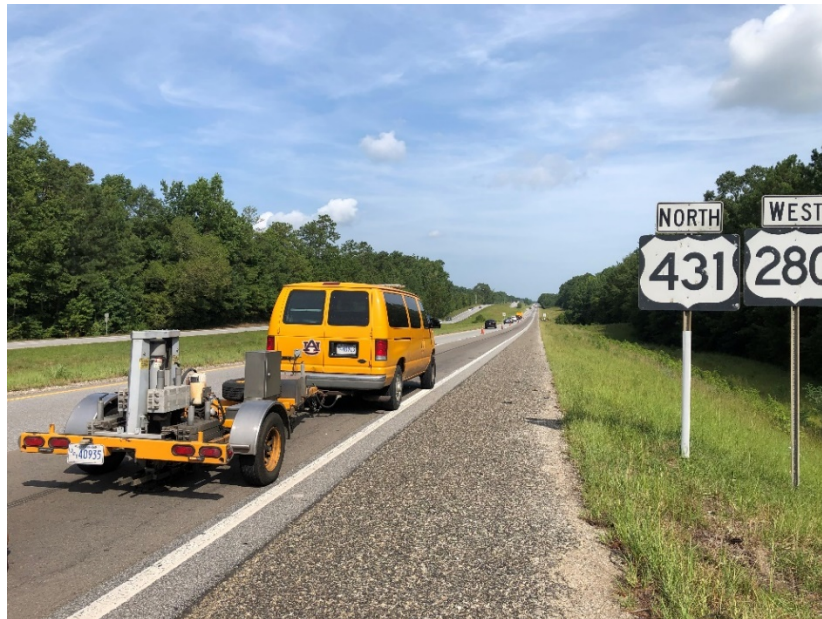
Figure 20. FWD testing on Highway US-280
