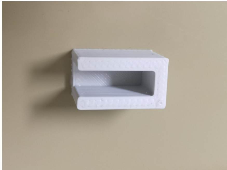
Figure 5.13: The box to hold the sample made by 3D printer.
