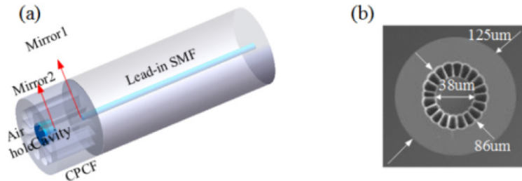
Figure 2.23: (a) A schematic diagram of an optical biosensor based on a concave-core PCF and FPI. (b) A microscope photograph of the cross section of the sensor. The concave-core forms a physically short cavity which allows liquid to flow into the sensor with ease and significantly reduces the measurement time. Reprinted from [22] with permission from OSA.
