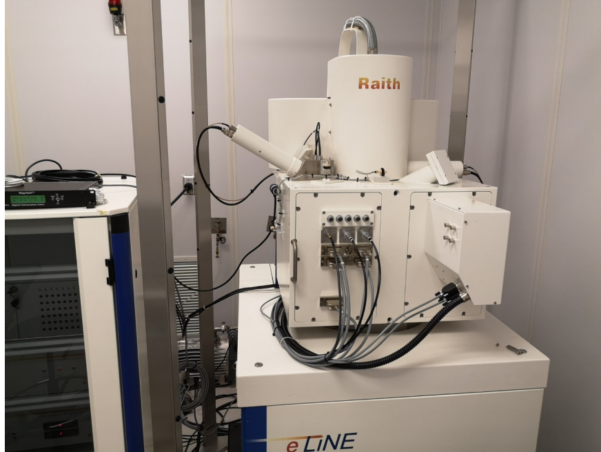
Figure 4.20: The image of A Raith TM 150 e-beam lithography system.
