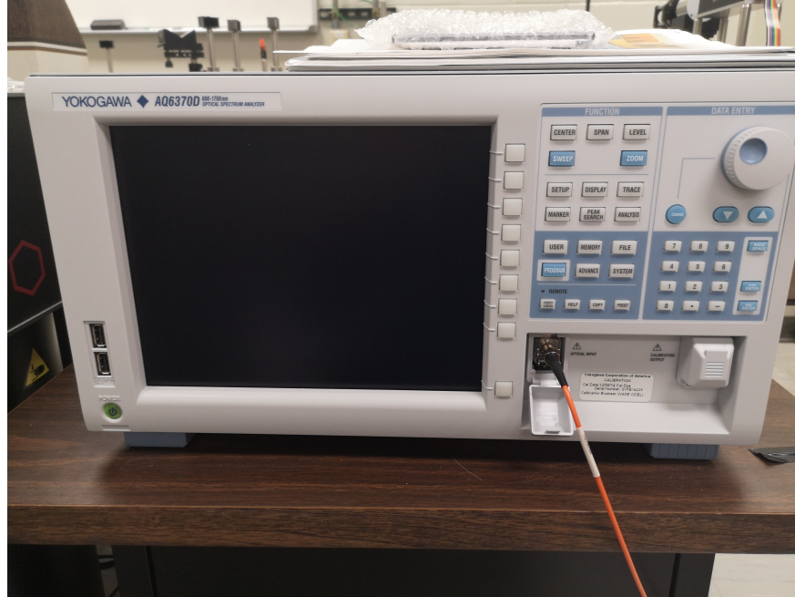
Figure 5.17: The spectrum analyzer (AQ6370D by Yokogawa) used in the experiment.
