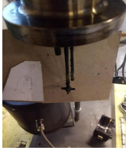
Figure 4.2 Product solidification and equipment corrosion during the upgrading of HTL oil alone
