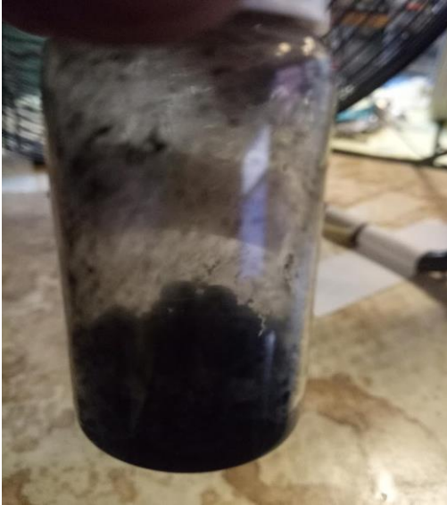
Figure 4.2 Product solidification and equipment corrosion during the upgrading of HTL oil alone
