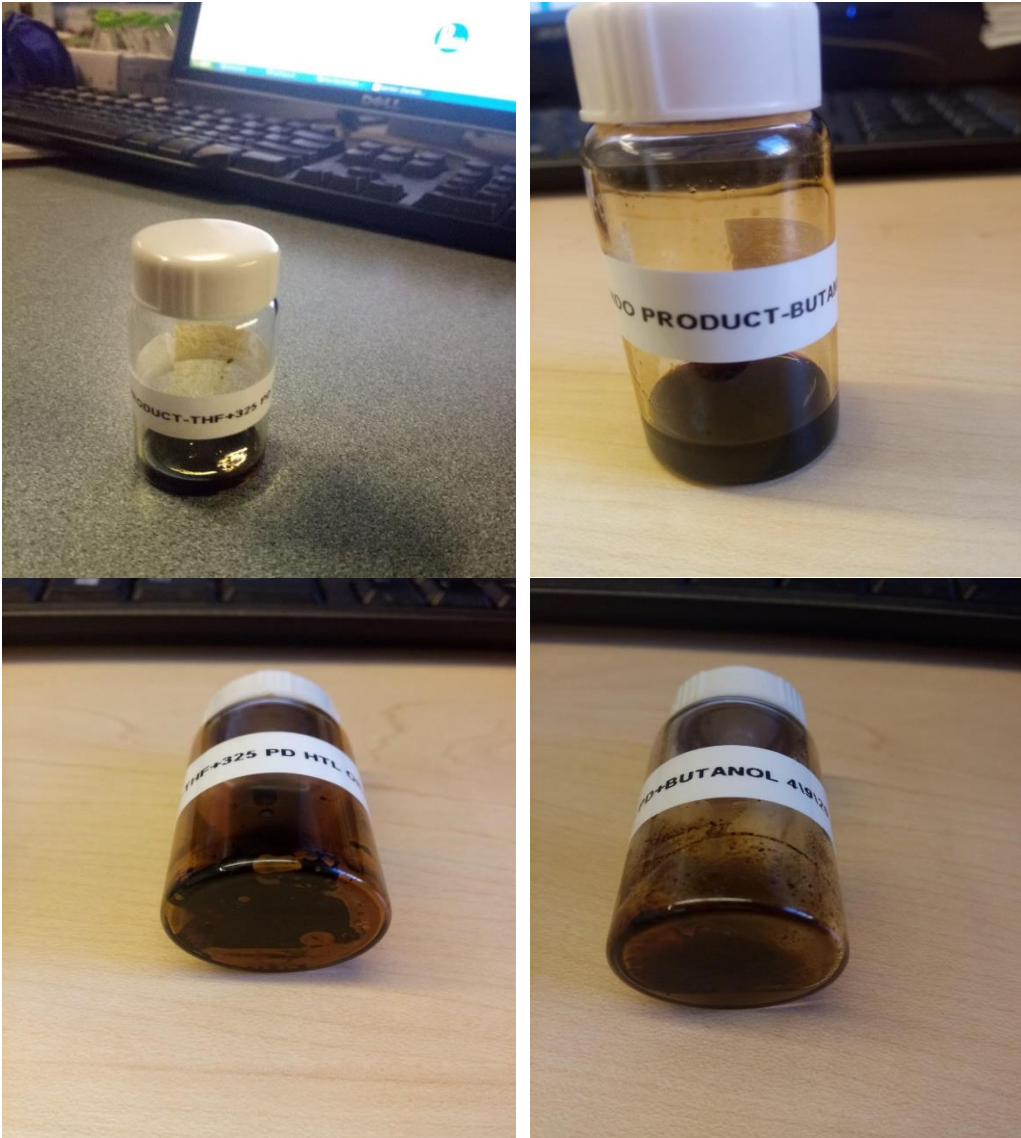
Figure A4.2 Liquid products from the hydrotreating of HTL oil in THF (left) and Butanol (right)
