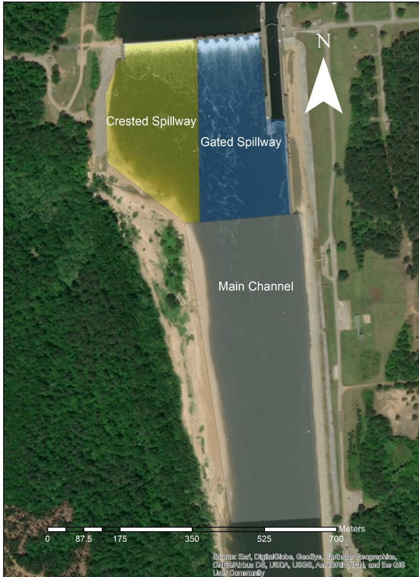
Figure 2. Habitat zones of Claiborne Lock & Dam tailrace. The crested and gated spillways are split down the middle of the whole tailrace. The main channel begins on the eastern shore at the edge of the long lock wall along rip rap and on the western shore where the sandy bank starts. It extends to the end of the rip rap and where the sandy bank becomes riverbank.
