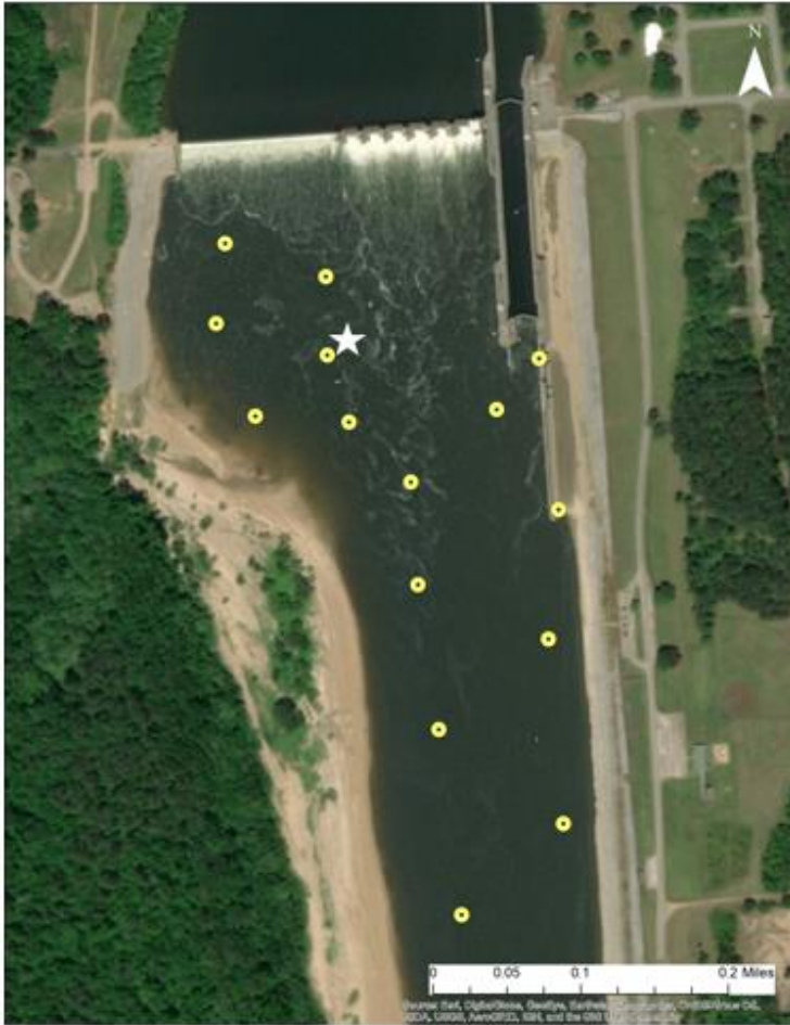
Figure 1. The array of 15 Lotek WHS 3250L series receivers located in the tailrace below Claiborne Lock and Dam. Each yellow circle represents the location of a single receiver. The star positioned between the crested spillway (left) and gated spillway (right) marks the release point of tagged fish.
