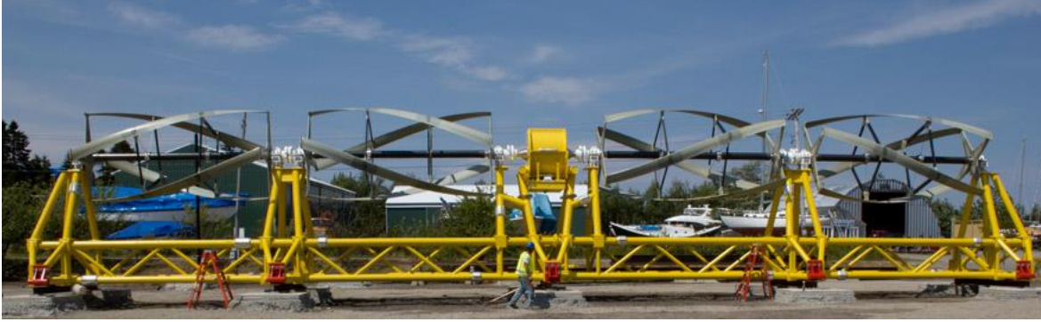
Figure 2.3. ORPC series-connected Gorlov turbine [23]
