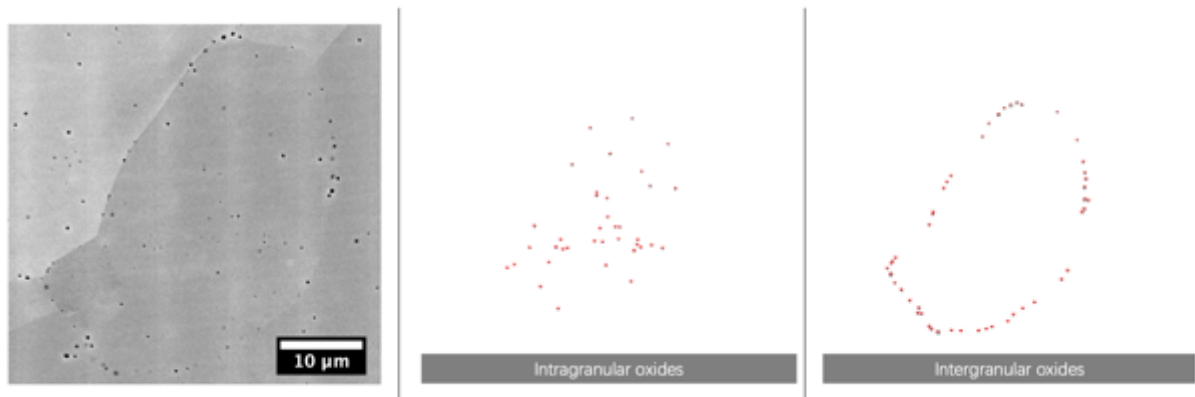
Fig 34 Example of analyzing volume fraction percent and number percent of intergranular and intragranular oxides using ImageJ.
