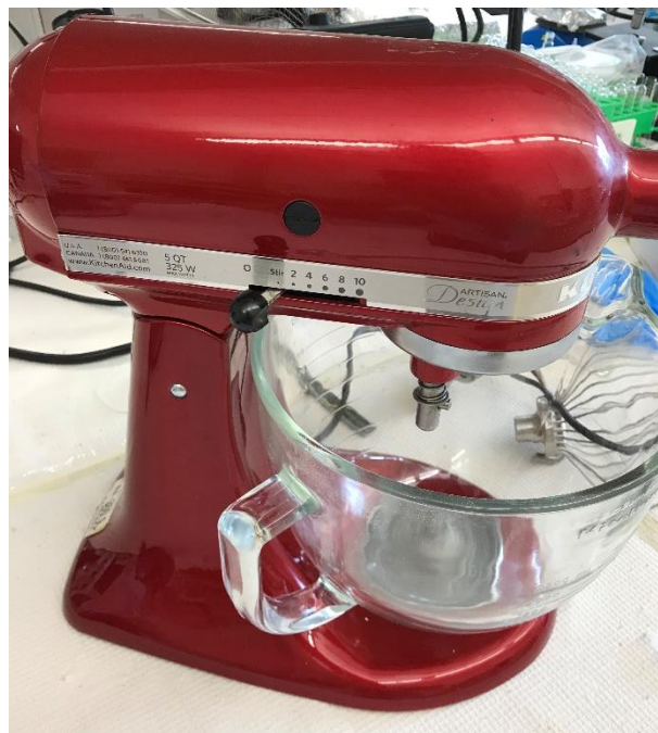
Figure 2-4 Blender used to mix the particleboard and the resin
