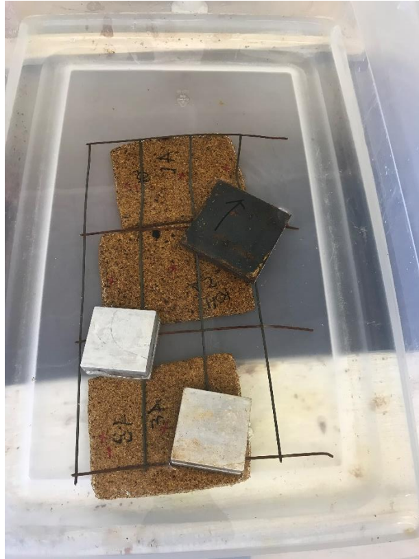
Figure 1-11: Samples soaked in water for TS, ES and WA determination
