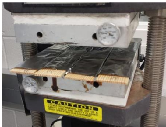
Figure 1-6: Hot press used for the lap shear test
