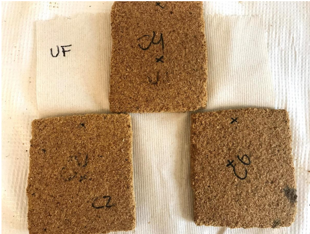
Figure 2-16: UF panels after soaking in water for 24hs for TS,ES and WA
