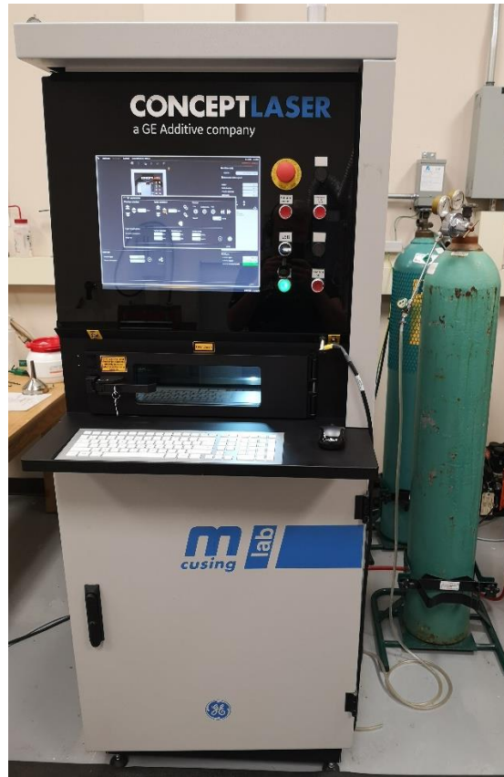
Figure 6: Picture of the Concept Laser MLab Cusing 100R L-PBF machine used for all AM processes
