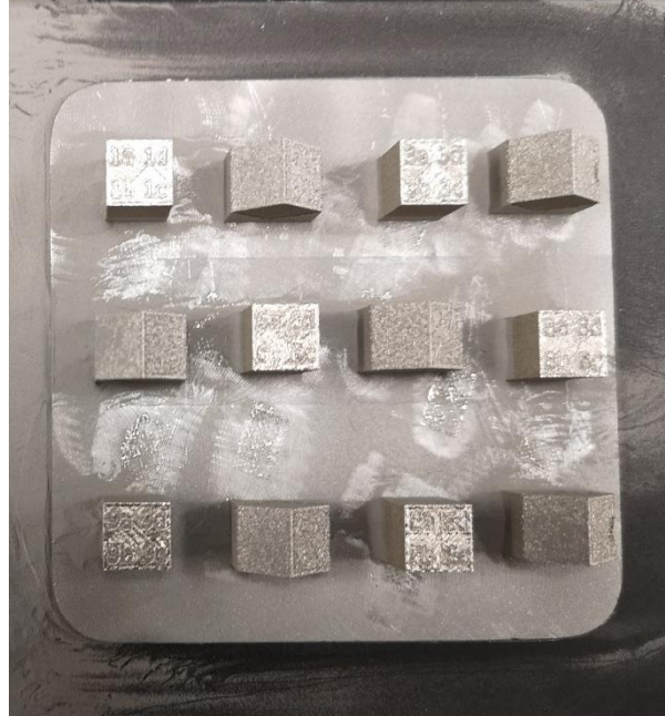
Figure 7: Arrangement of the manufactured INC625 cubes on the built plate
