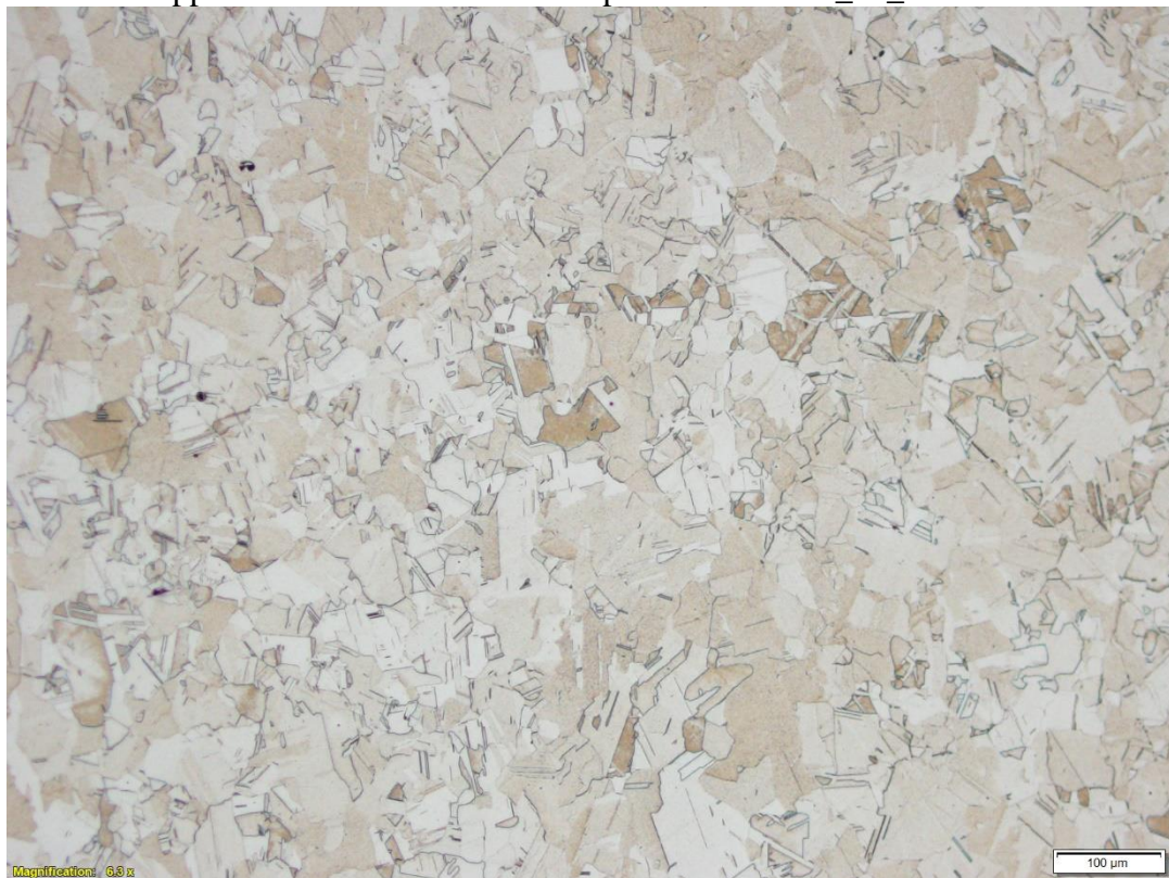
Appendix D: Microstructure of specimen 1050°C_1h_V
