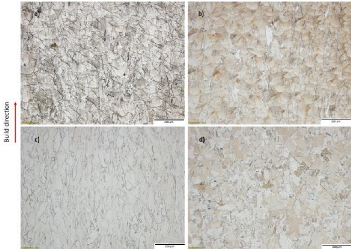
Figure 11: Microstructure of AM IN625 a) As-built condition, b) heat treated at 700°C for 1 hour, air cooled, c) heat treated at 900 °C for 1 hour, air cooled, d) heat treated at 1050 °C for 1 hour, air cooled.
