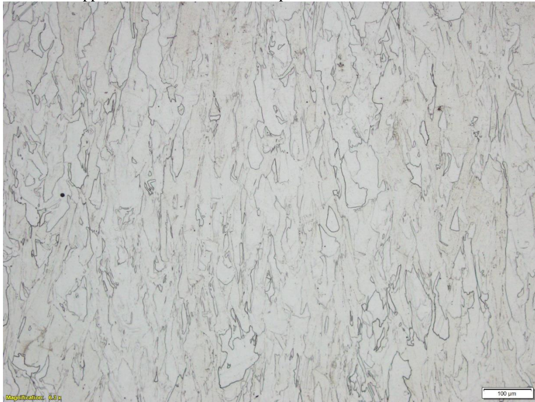
Appendix D: Microstructure of specimen 1050°C_1h_V
