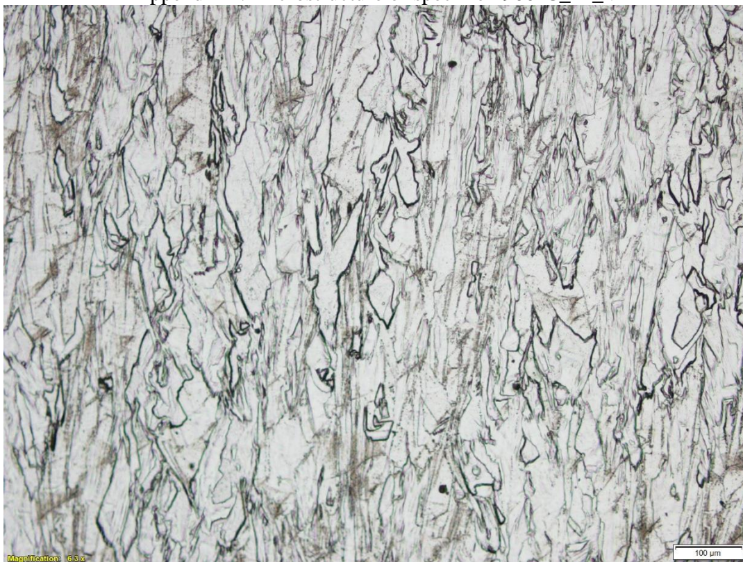
Appendix F: Microstructure of specimen 900°C_1h_V
