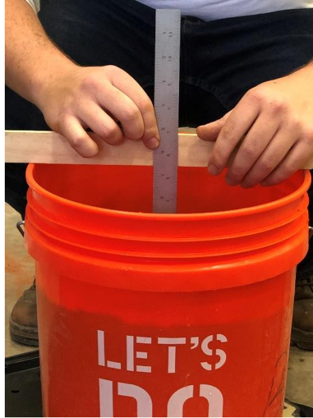
Figure 3.19: Height measurement of DCP specimen
