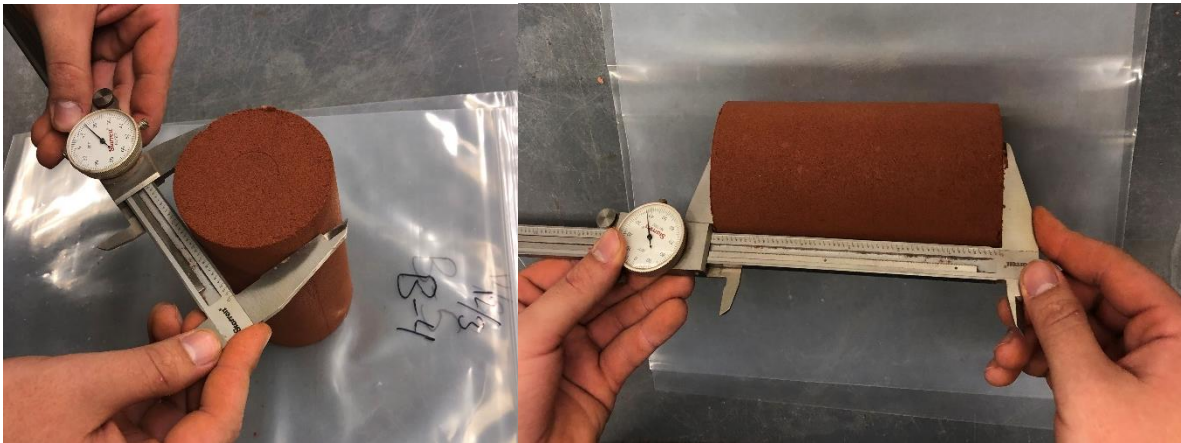
Figure 3.15: Measurements of the soil cement cylinder using a caliper
