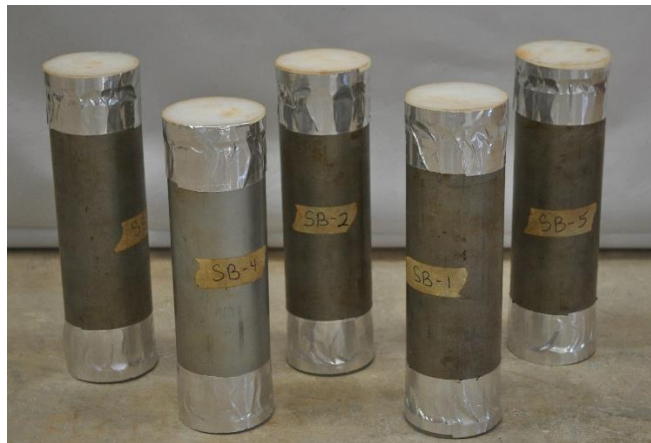
Figure 2.49: SM cylinders during initial curing period
