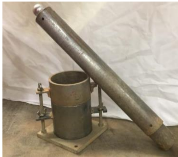
Figure 2.41: Proctor mold and 5.5-pound hammer
