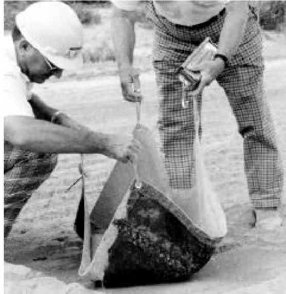
Figure 2.19: Cement content being checked (ACI 230 2009)
