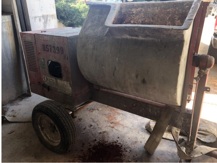
Figure 3.8: 12-cubic foot mortar mixer for soil cement mixing
