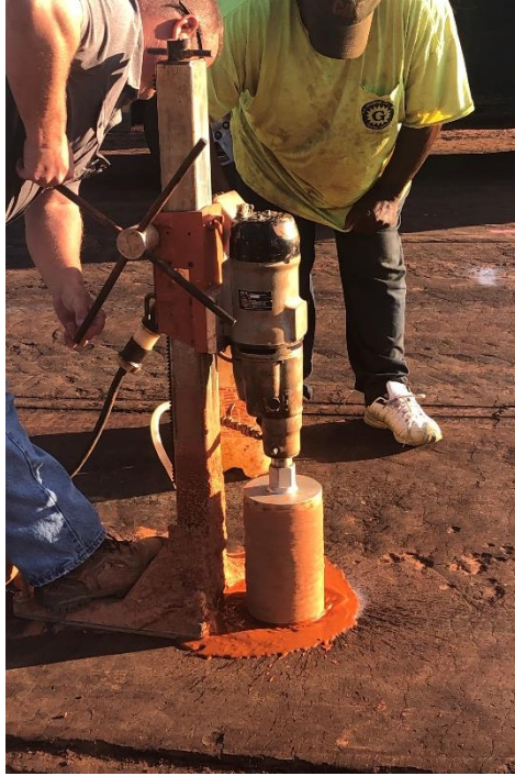
Figure 3.33: Core being recovered from the section
