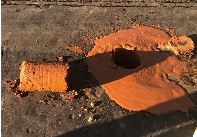
Figure 2.24: A sampled core that is too small
