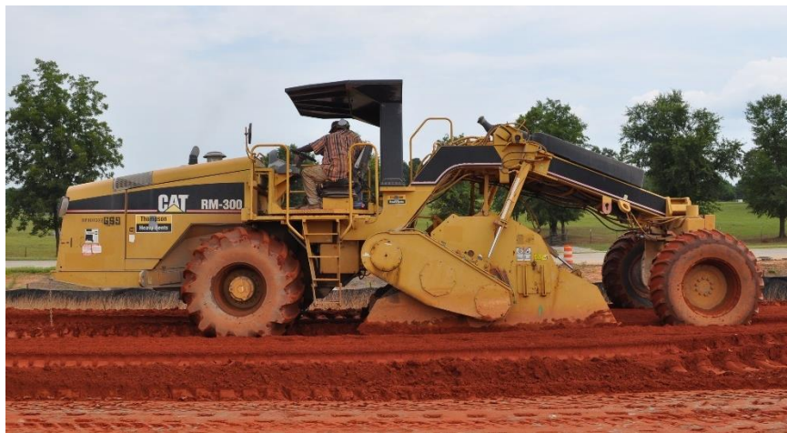
Figure 2.10: Transverse single-shaft mixer
