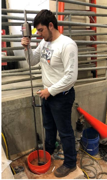
Figure 3.21: DCP testing arrangement in the specimen
