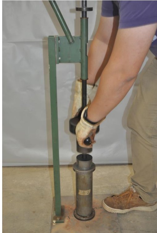
Figure 2.48: SM cylinder compacted with drop-weight machine
