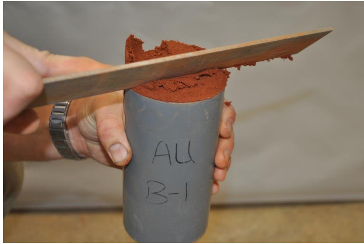
Figure 3.11: Straightedge used to trim the soil cement to the top of the mold
