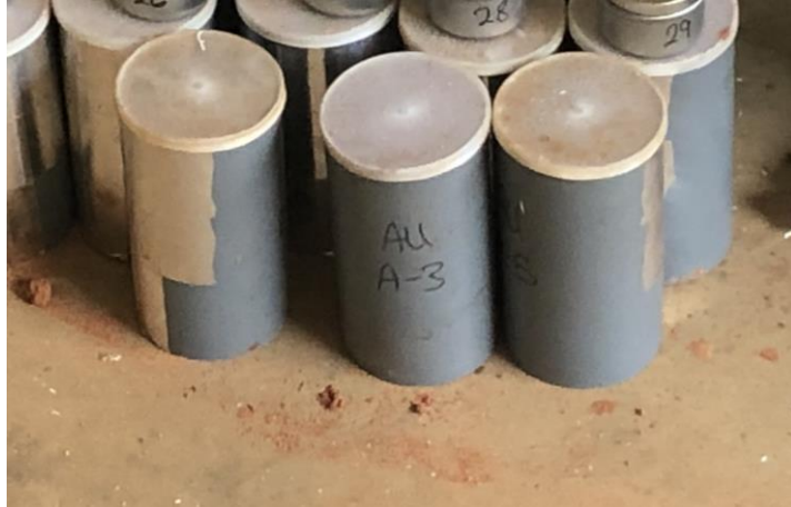
Figure 3.28: PM specimens during initial curing on site
