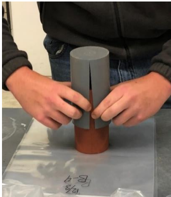
Figure 3.12: Specimen removal from plastic-mold
