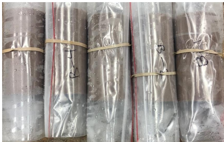
Figure 3.14: Final curing of the PM cylinders
