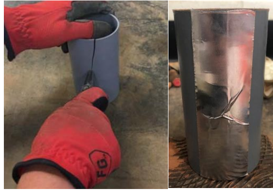
Figure 2.45: Plastic mold modification process (McLaughlin 2017)
