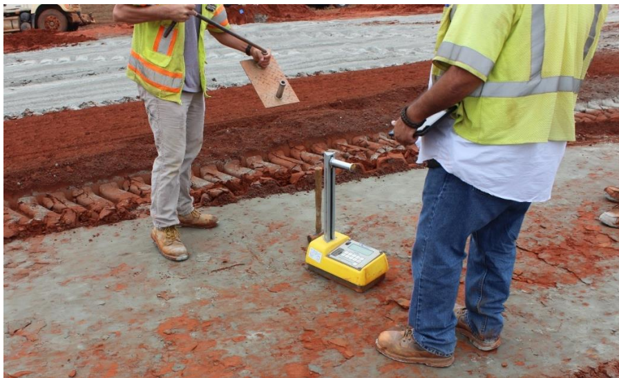
Figure 2.20: Nuclear gauge method right after rolling
