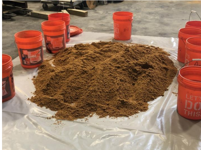
Figure 3.7: Mixing of soil prior to batching
