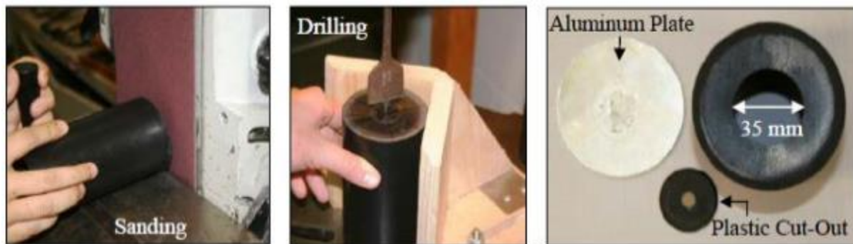
Figure 2.43: Plastic mold modification (Sullivan et al. 2014)
