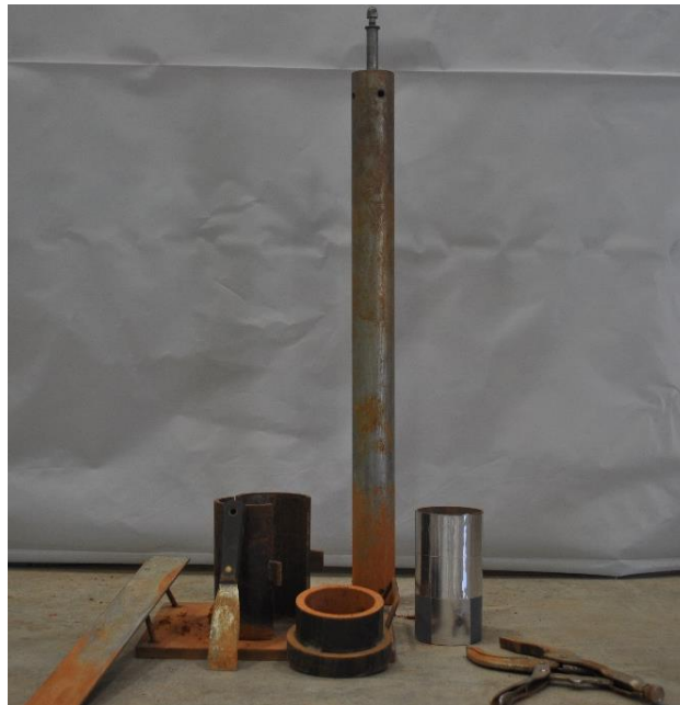
Figure 2.42: Plastic-Mold preparation apparatus
