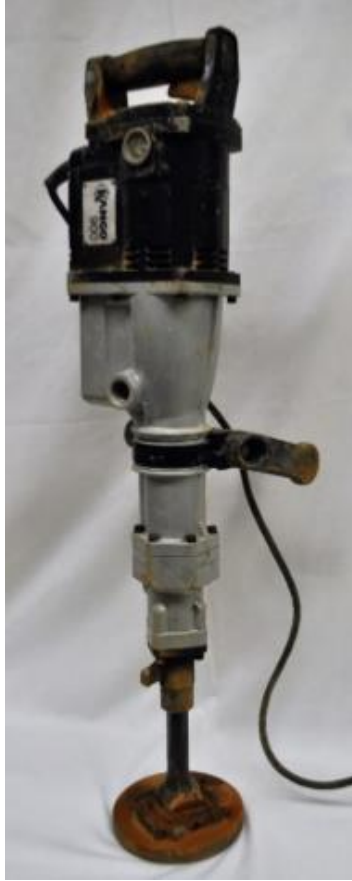
Figure 2.32: Vibrating compaction hammer with circular steel plate
