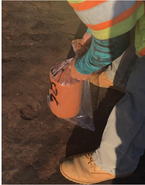
Figure 3.34: Core being placed in plastic bag
