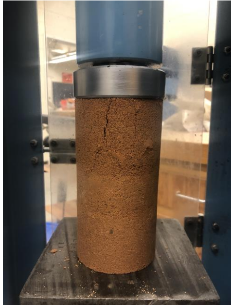
Figure 3.18: Specimen being tested in the 100-kip compression testing machine
