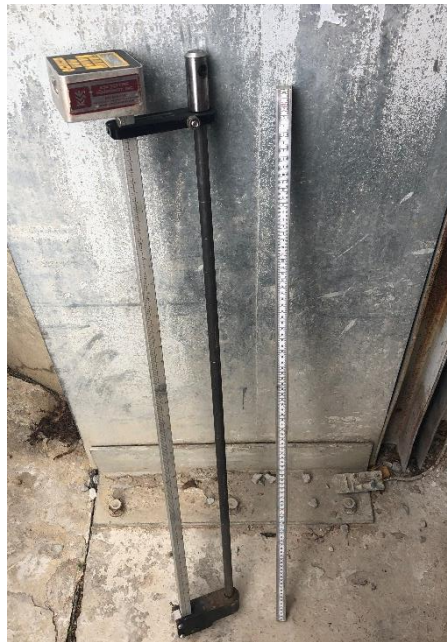
Figure 3.32: Magnetic ruler and manual ruler used for DCP testing
