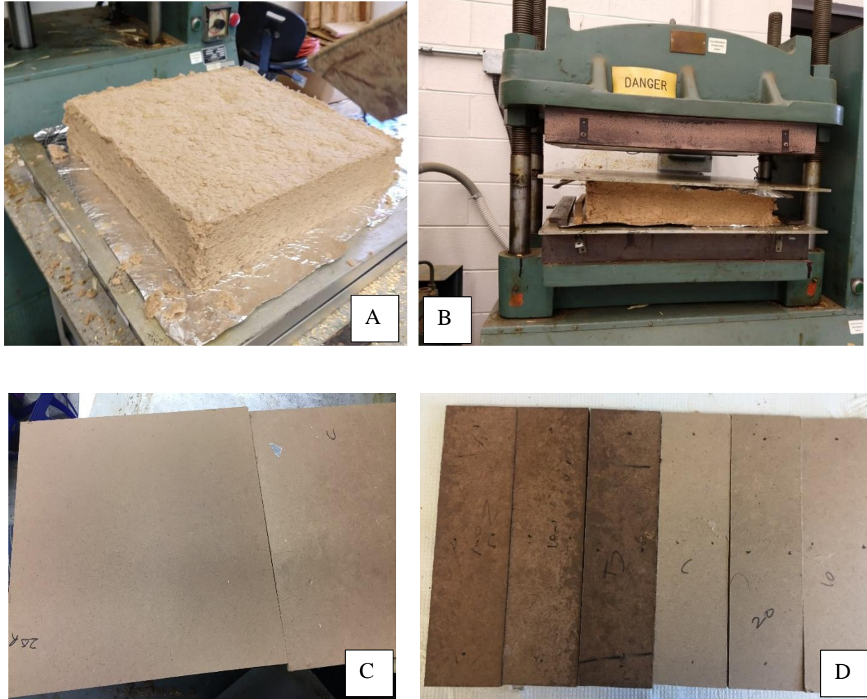
Figure 7.1: 1 Medium density fiber board mat (A); hot press with MDF mat (B); trimmed MDF panels (C); Tested specimen for MOR and MOE (wet from left (dark colored) and dry) (D).
