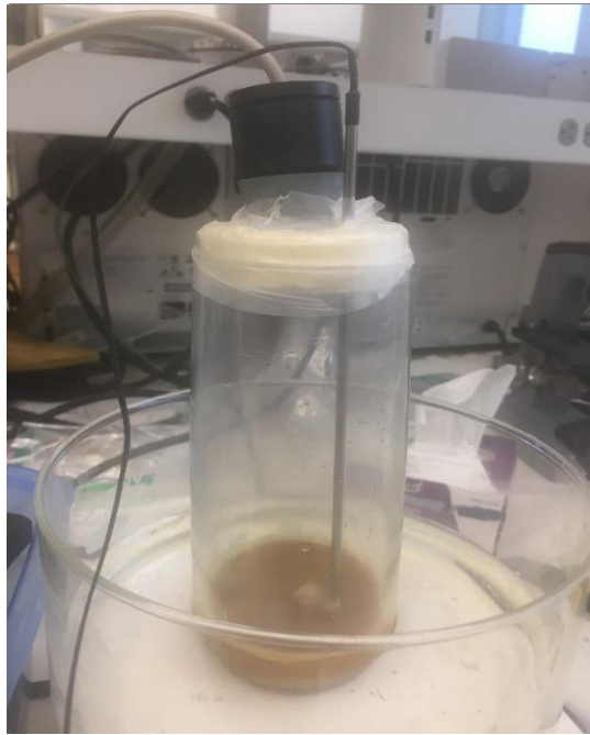
Figure 7.2: CO 2 measurement set up with a thermometer and CO 2 sensor housed in the cover.
