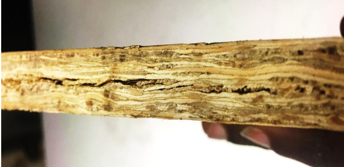
Figure 5.5: Delaminated OSB panel pressed for 1.5 minutes.
