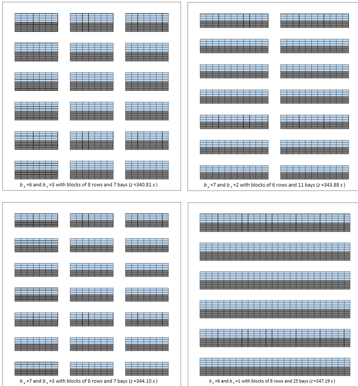
Figure 5.15. The remaining four best layout configurations along with cycle times for \delta_x = 2 bays and \delta_y = 5 rows
