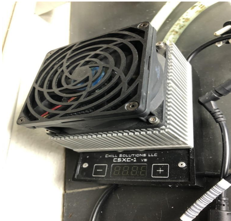
Figure 11. The adjustable thermostatic constant temperature chillers CSXC-1, showing the fan and chiller heat exchanger. (Chill Solution LLC.)
