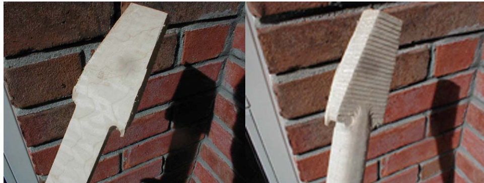
Figure 3.30 The headstock following CNC routing.
