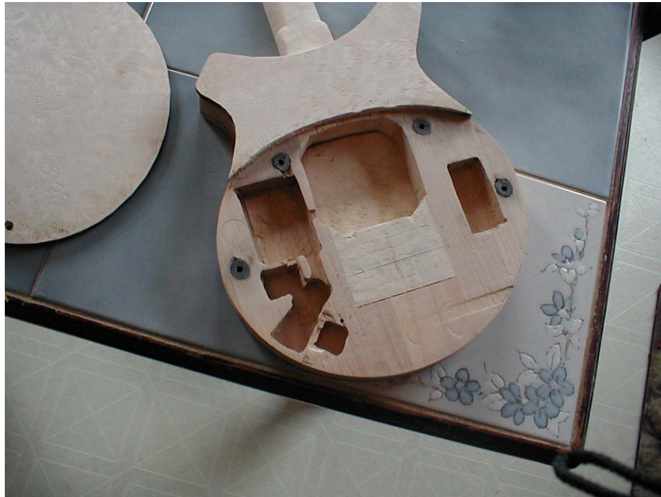
Figure 3.37 Cavities created to contain electronic components.
