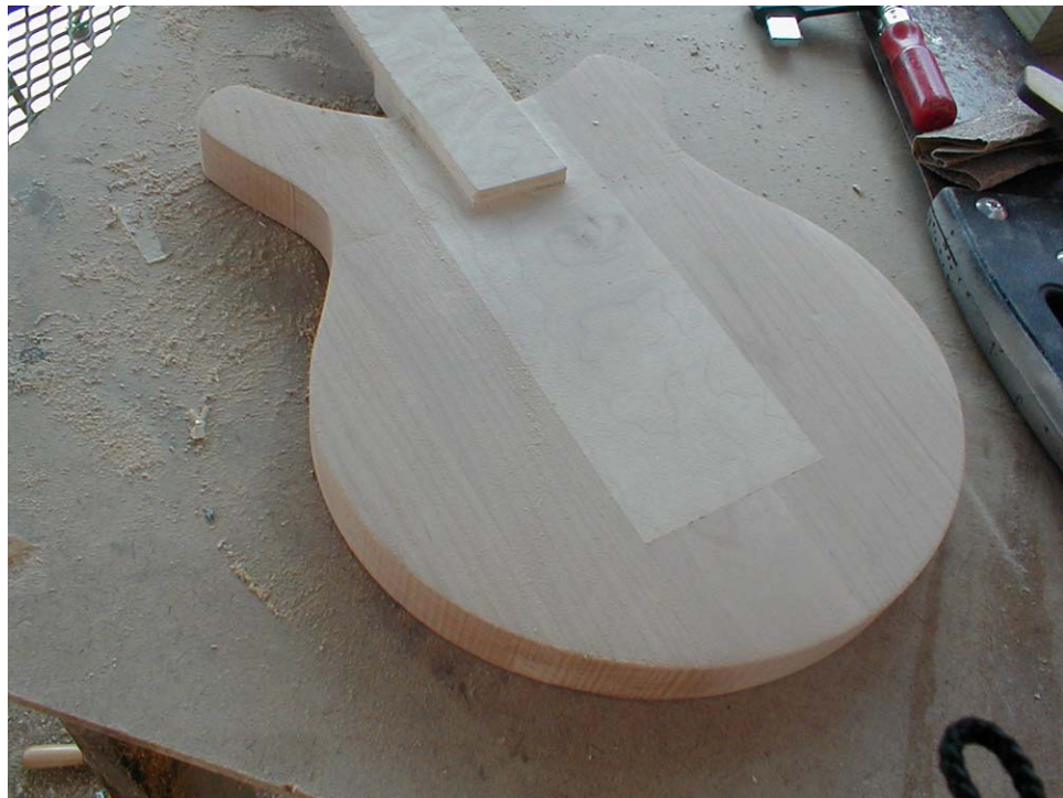
Figure 3.33 The body routed down one quarter of an inch.
