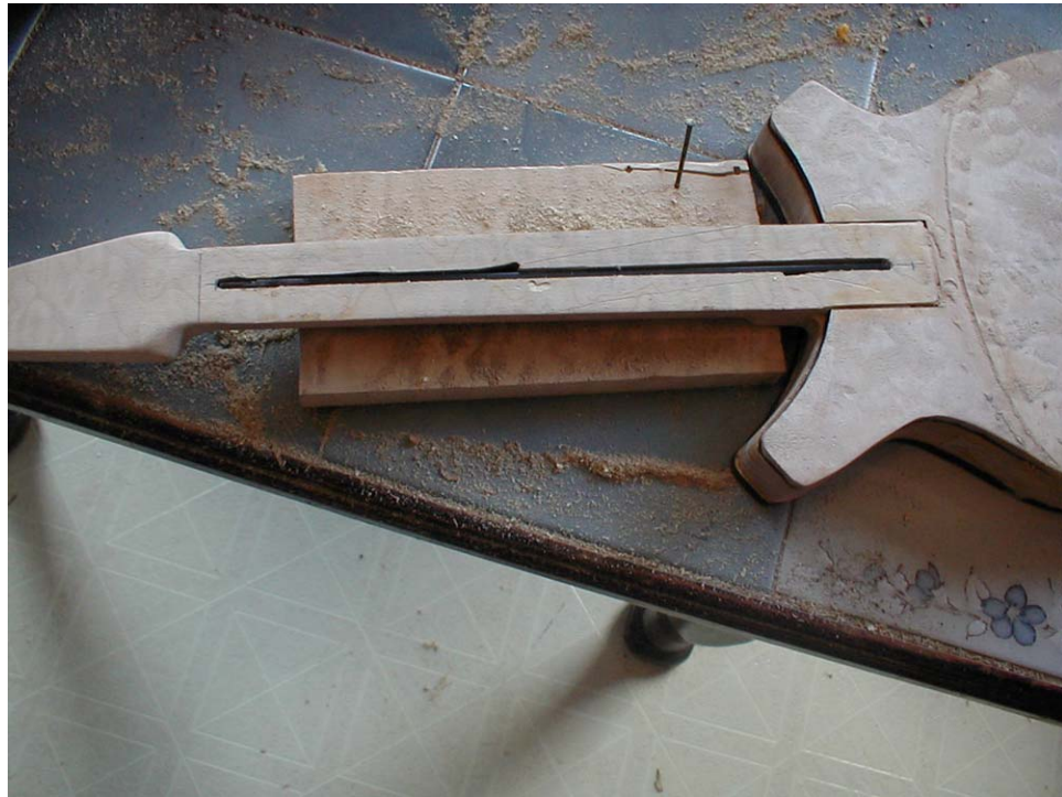
Figure 3.39 The truss rod after being set into its slot, prior to gluing.
