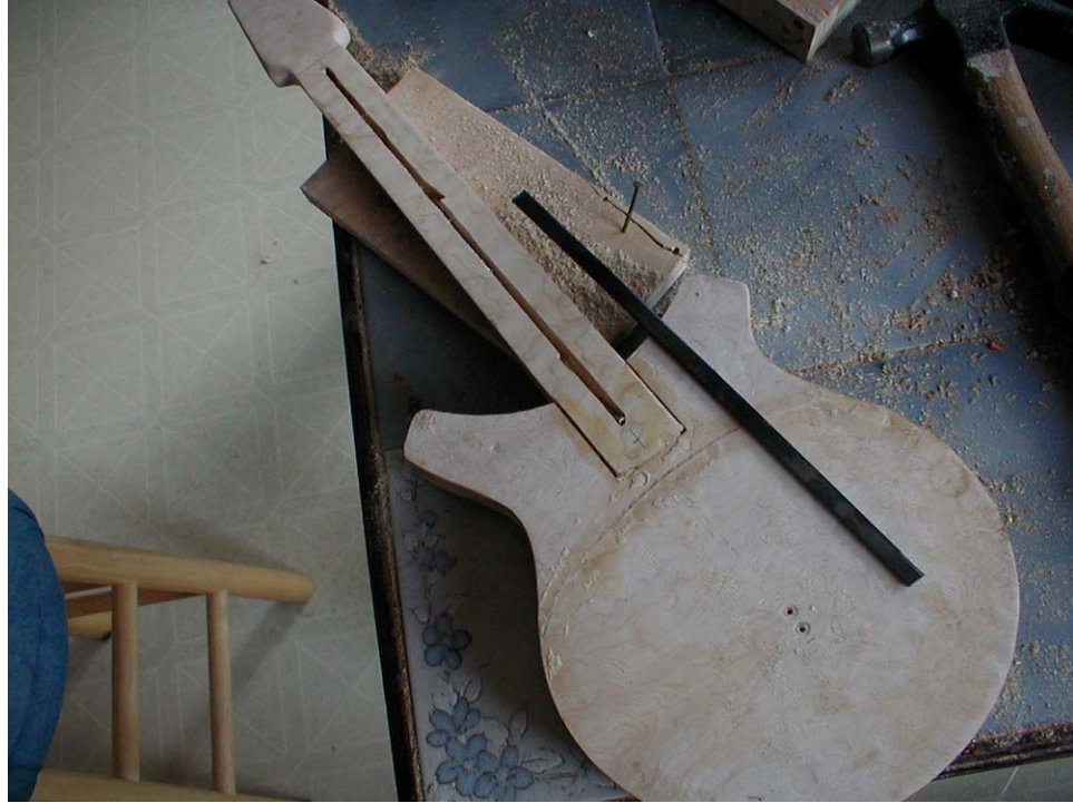
Figure 3.38 Routed half inch slot and carbon fiber truss rod.
