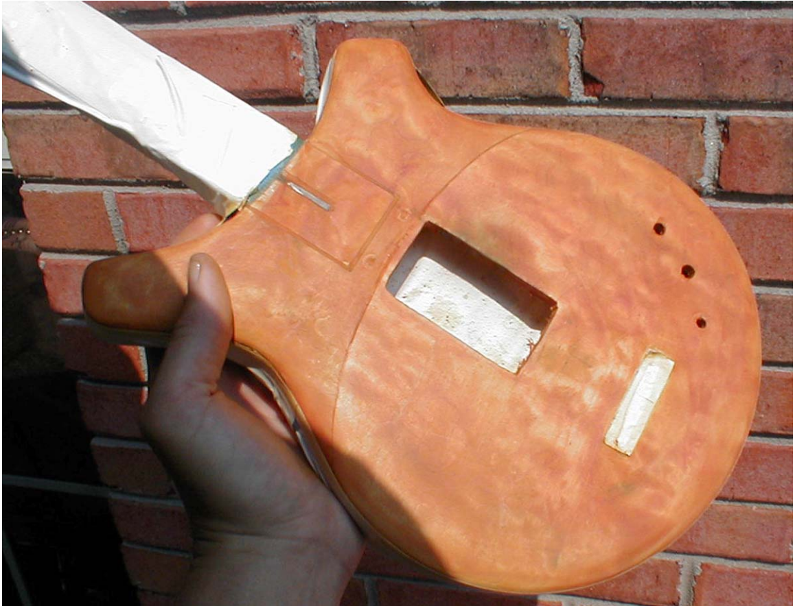
Figure 3.43 Guitar body following sanding the first aniline dye application.
