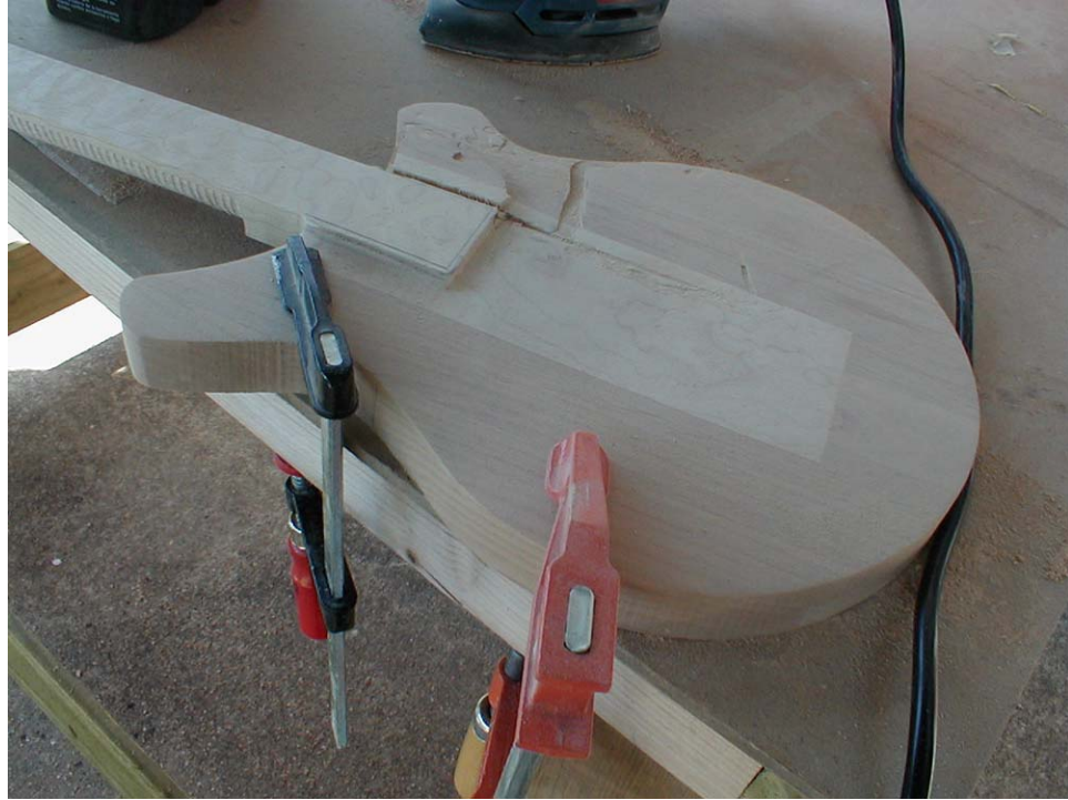
Figure 3.32 Routing down the top of the body to accommodate the maple tops.
