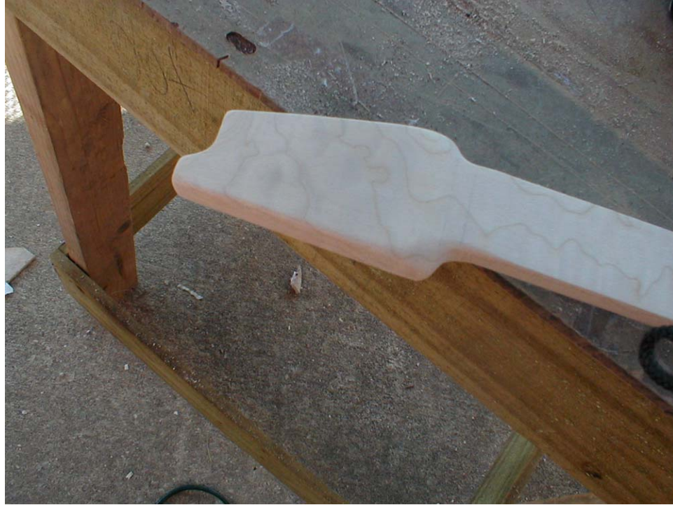
Figure 3.31 The headstock after being hand shaped into its final form.
