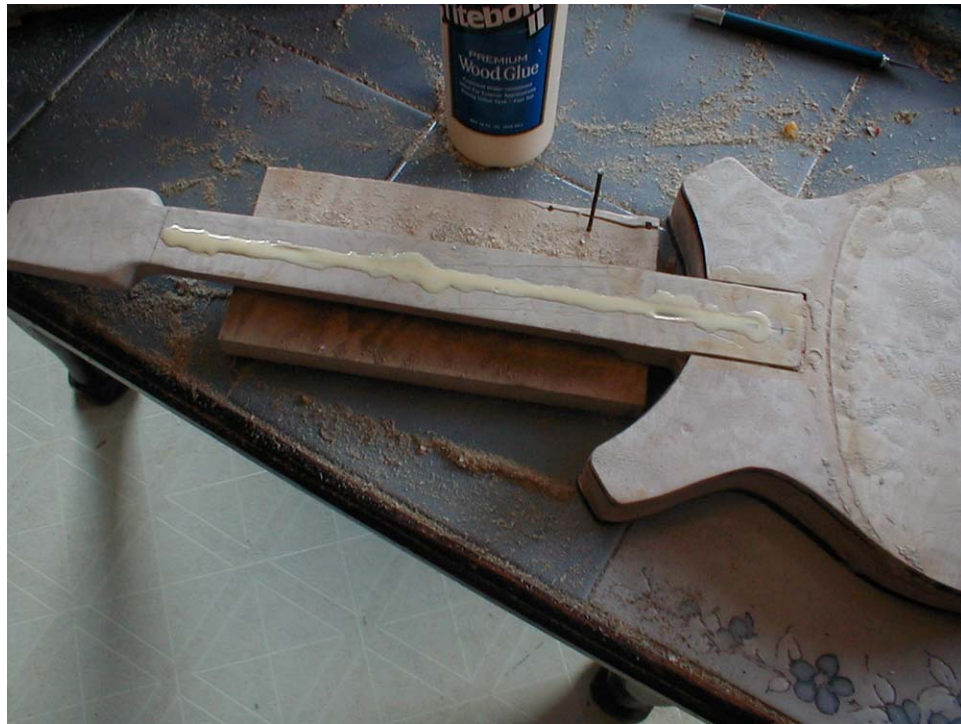
Figure 3.40 Gluing the carbon fiber truss rod into its slot with wood glue.
