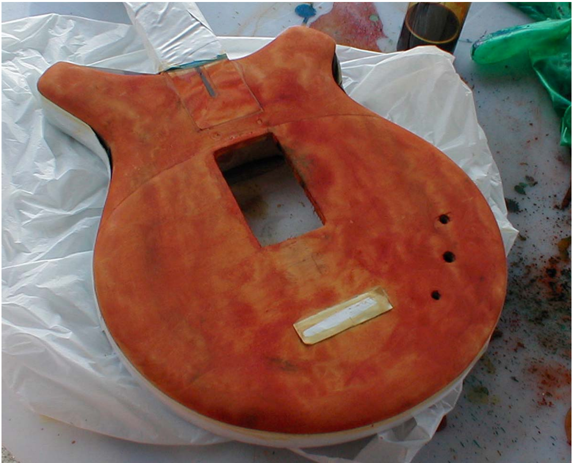
Figure 3.44 Guitar body following the second aniline dye application.
