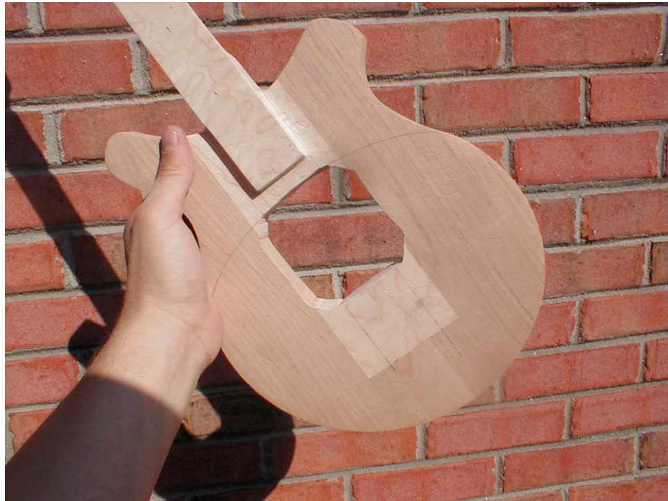
Figure 3.35 The completed speaker hole.
