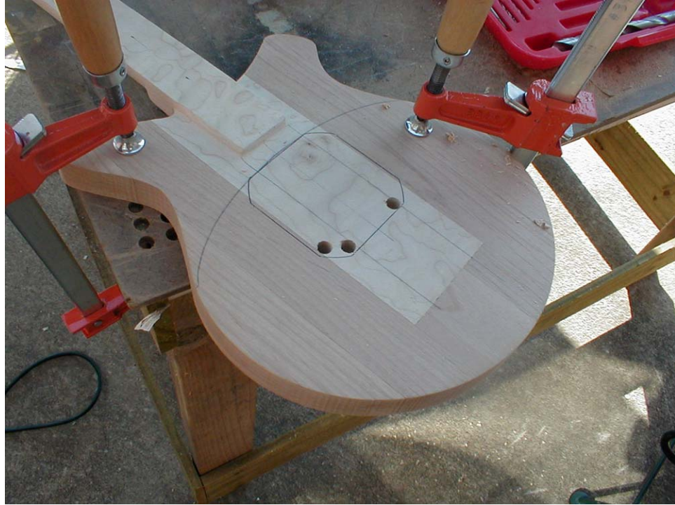
Figure 3.34 Preparing to cut the speaker hole by creating access holes for the jig saw.
