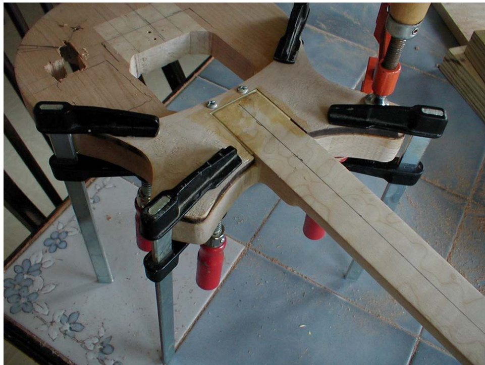
Figure 3.36 The forward section of the front maple top being glued onto the body.
