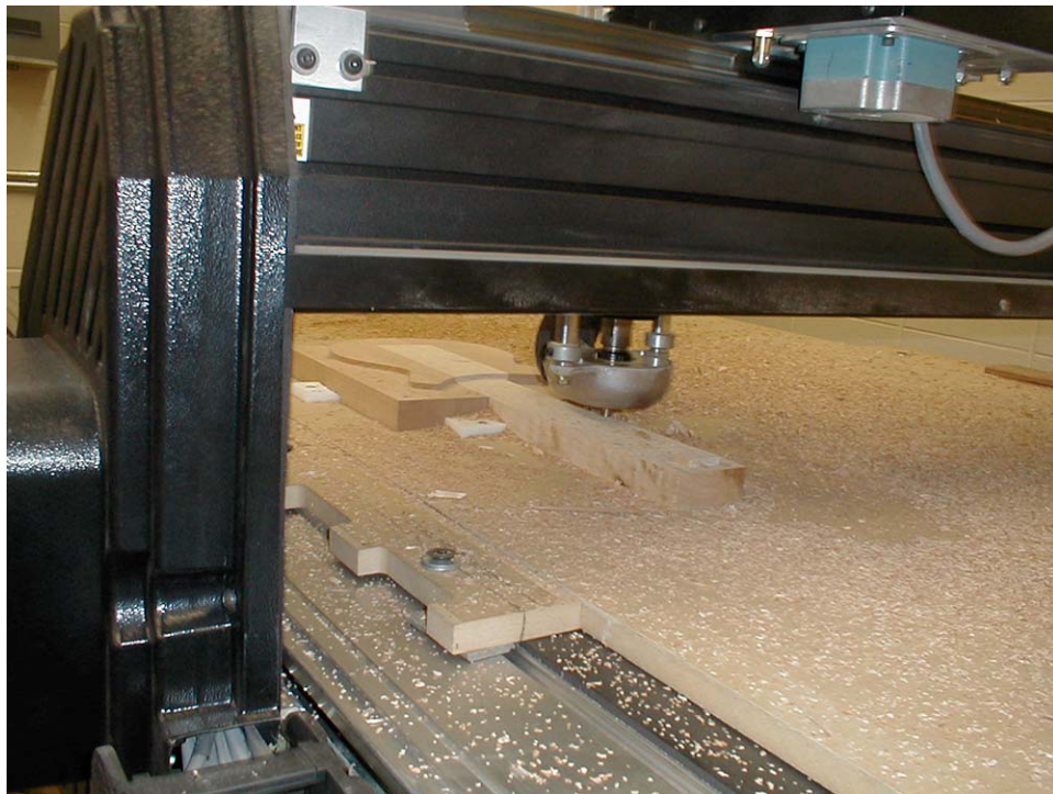
Figure 3.26 Alder and maple block being formed by the CNC Router.
