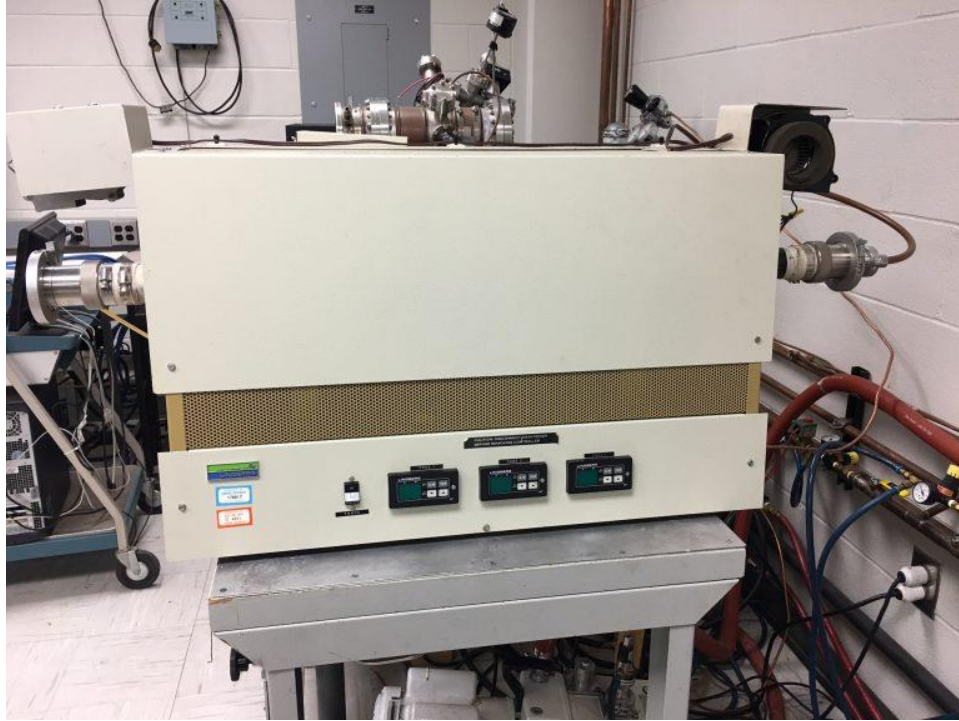
Figure 2.2. The three-zone tube furnace that is used for thermal treatments.
