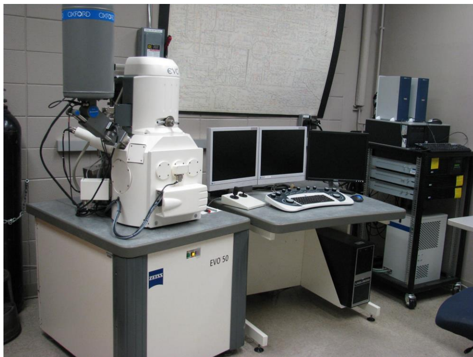
Figure 2.4. The SEM system that is used to analyze the topography and structural composition of the deposited samples.
