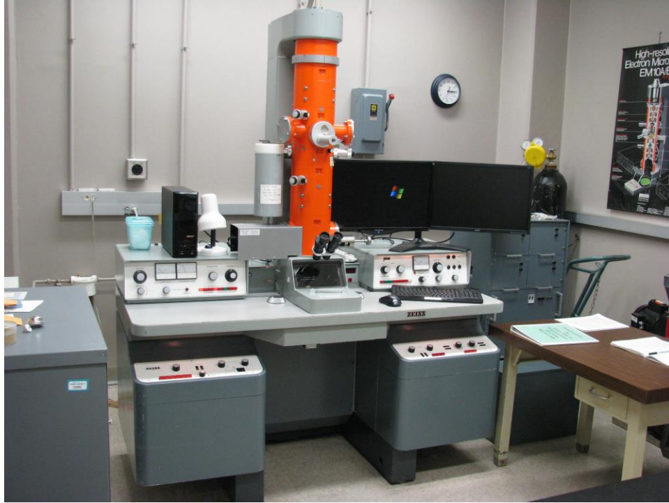
Figure 2.5. The TEM that is used to characterize single-particle and aggregation.
