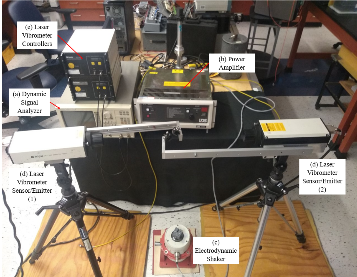
Figure 4.22: Test equipment used for during transmissibility analysis of fabricated MVIs.
