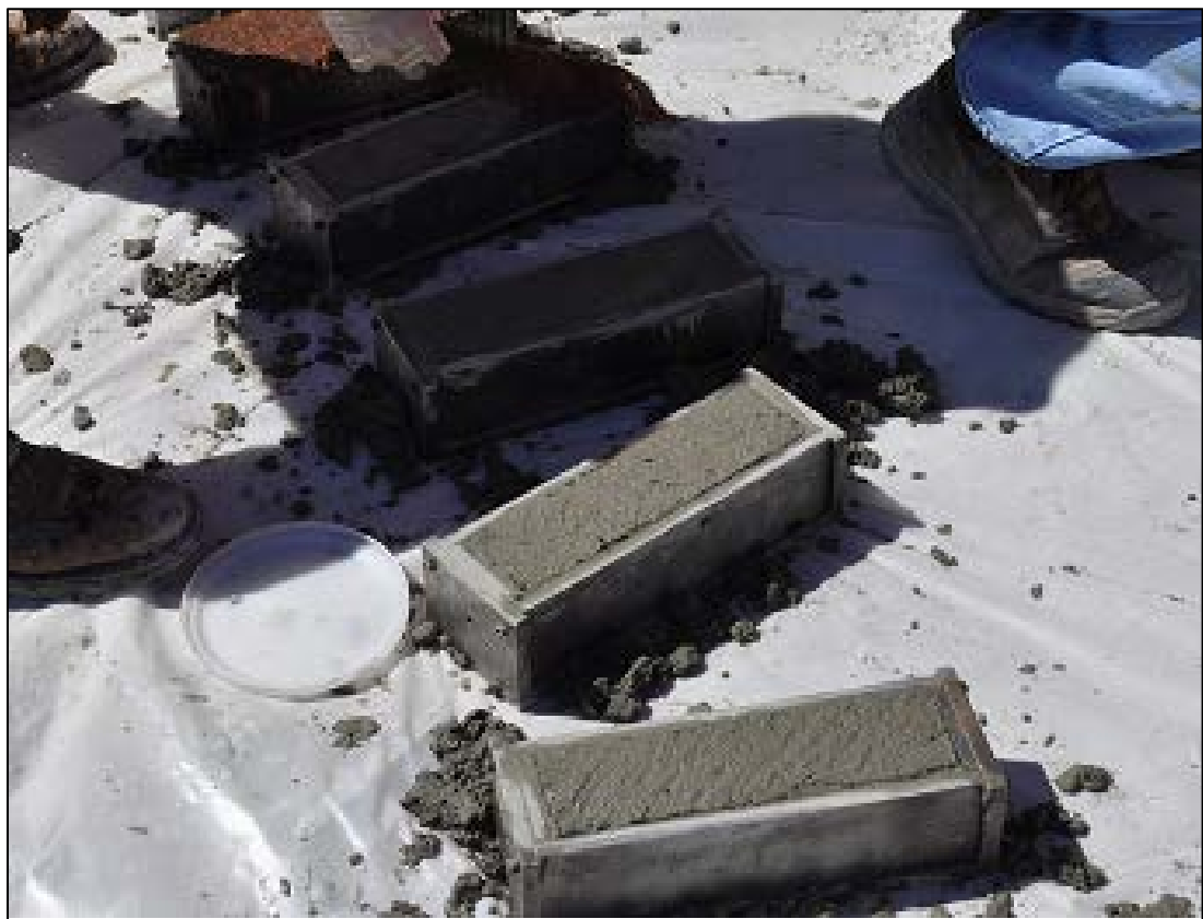
Figure 3-5: Concrete prisms being prepared at the jobsite
