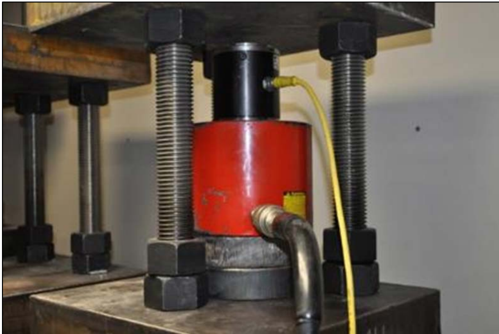
Figure 3-13: Standard setup of hydraulic ram and load cell used to apply stress
