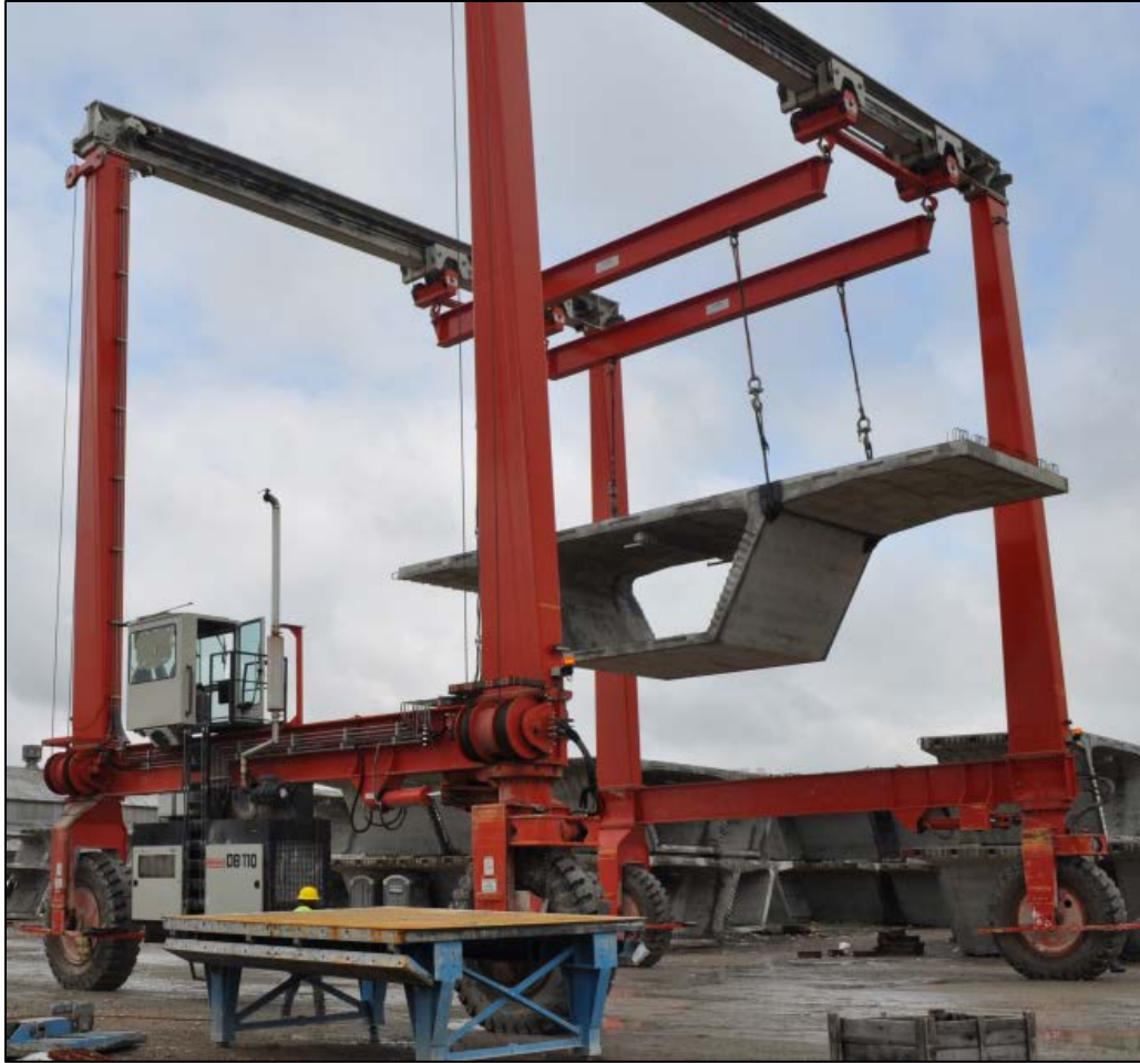
Figure 4-14: Rubber-tired gantry crane used to transport segments around the casting yard
