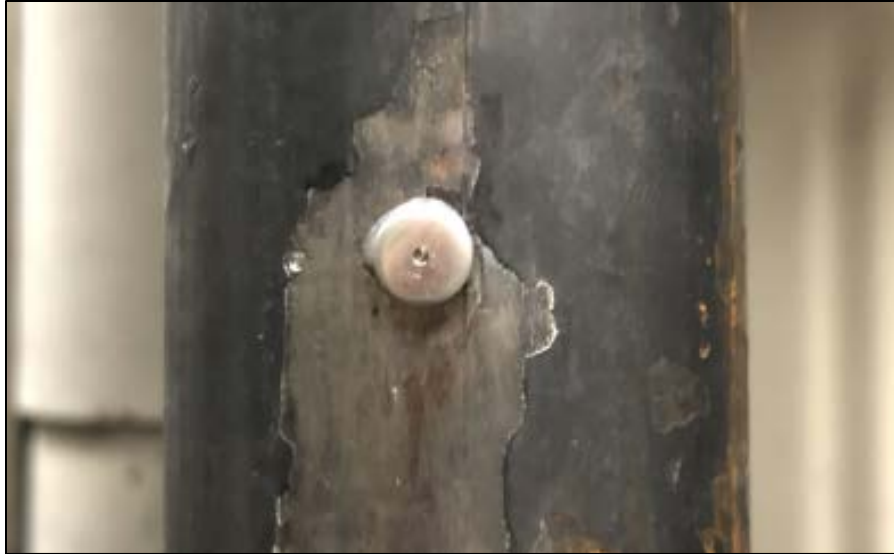
Figure 3-17: Epoxied DEMEC point on steel bar for load calculation
