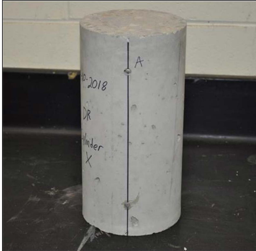
Figure 3-10: DEMEC points fixed to a concrete cylinder
