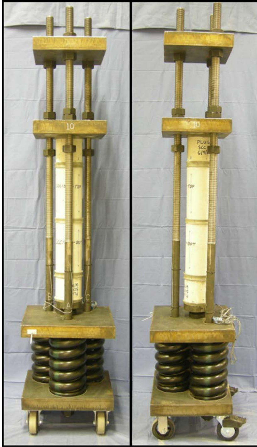
Figure 3-14: Creep frame used for testing at Auburn University (Kavanaugh 2008)
