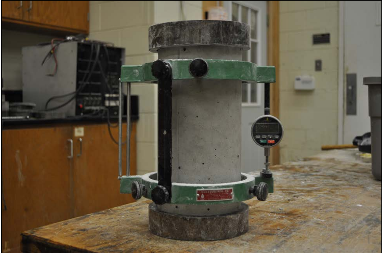
Figure 3-8: Compressometer used to test modulus of elasticity
