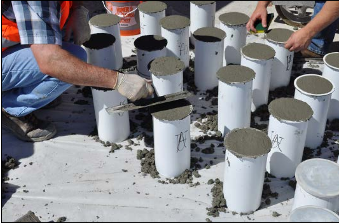
Figure 3-4: Concrete cylinders being prepared at the jobsite
