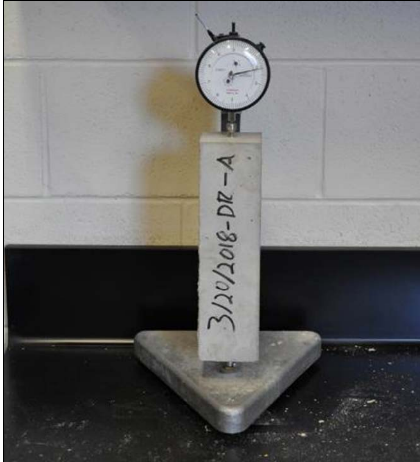
Figure 3-9: Standard length comparator used to measure drying shrinkage
