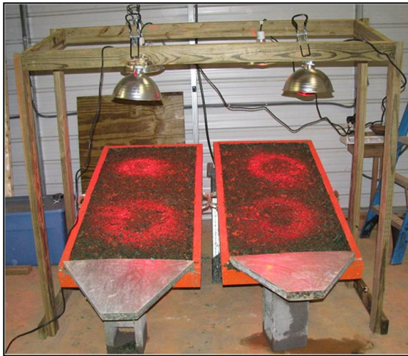
(a) Drying of Test Plots during Hydromulch Testing
