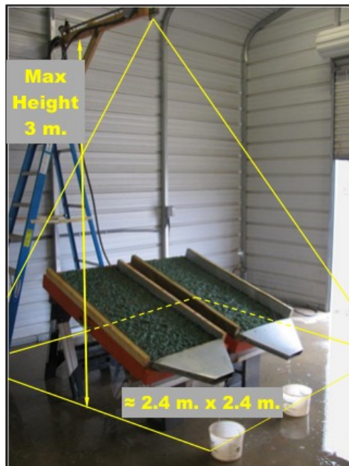
Figure 2-1 Illustration of Rainfall Simulator and Small-Scale Test Plots (Wilson 2010)
