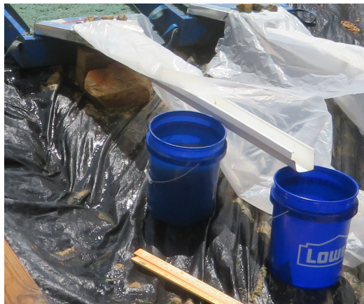
Figure 3-17 Runoff Collection Device for Small- and Intermediate-Scale Test Plots
