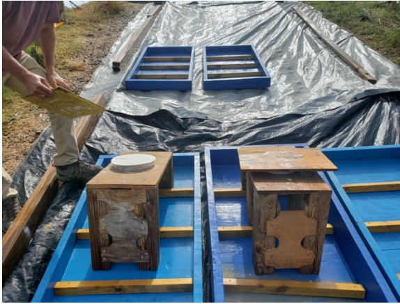
(a) Drop Size Collection Setup Using Flour Pan Method
