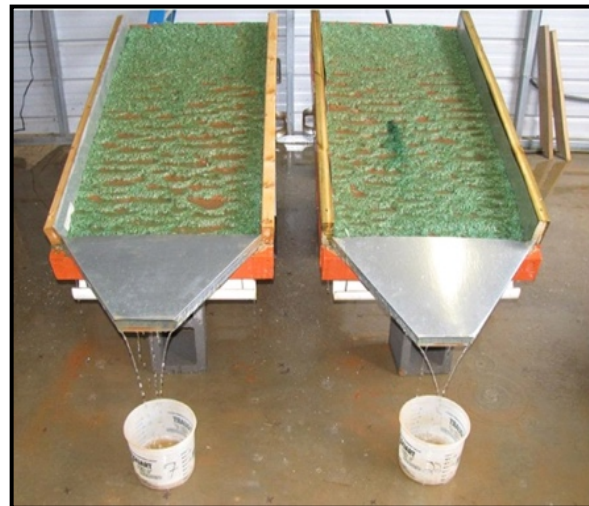
(b) Collection from Runoff for Each Test Plot
