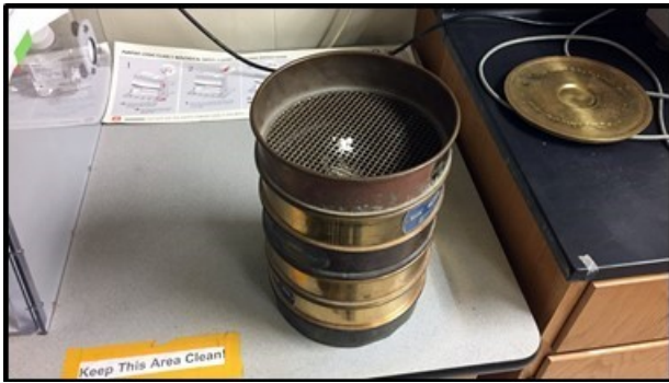
(c) Separating Pellets in a Sieve Stack;
