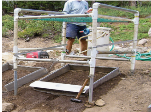
(b) Typical Small-Scale Rainfall Simulator (Grismer 2012)
