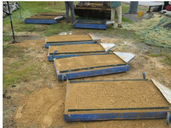
(b) Scarify Surface of Small-Scale Test Plots.
