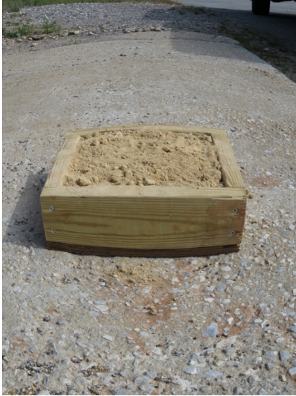
(a) Soil Compaction Testing Box;
