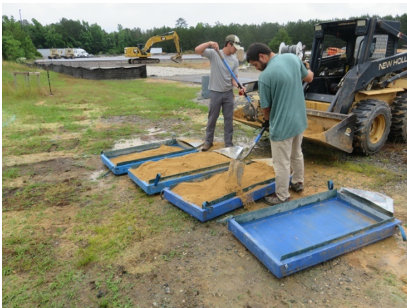
(a) Filling of Small-Scale Test Plots;
