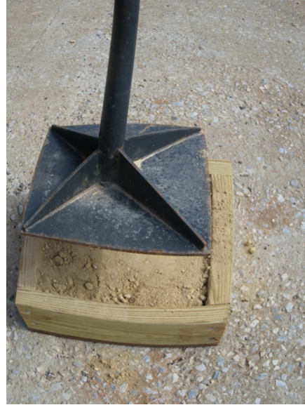
(b) Hand Tamper for Soil Compaction Testing.
