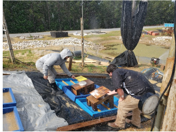
(b) Drop Size Collection Using Flour Pan Method
