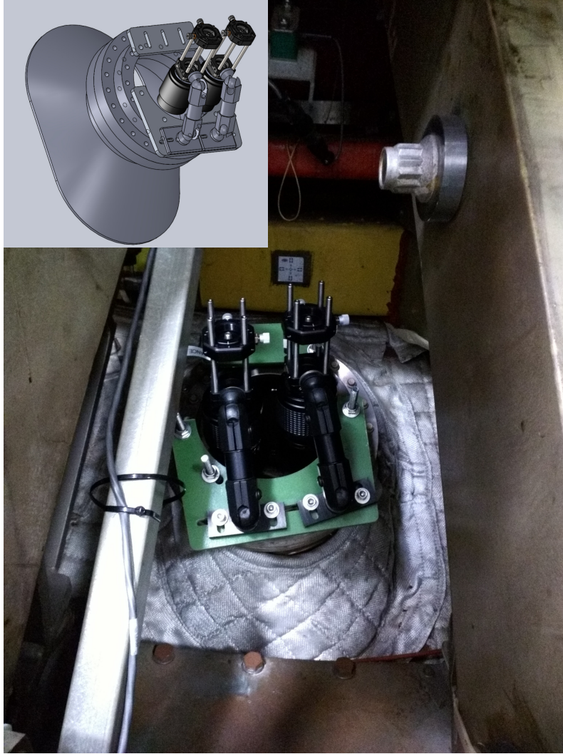
Figure 2.2: Mechanical drawing of collection optics and photo of collection optics installed on DIII-D. at a toroidal angle of 75^\circ and poloidally near the top of the machine (75R+2).
