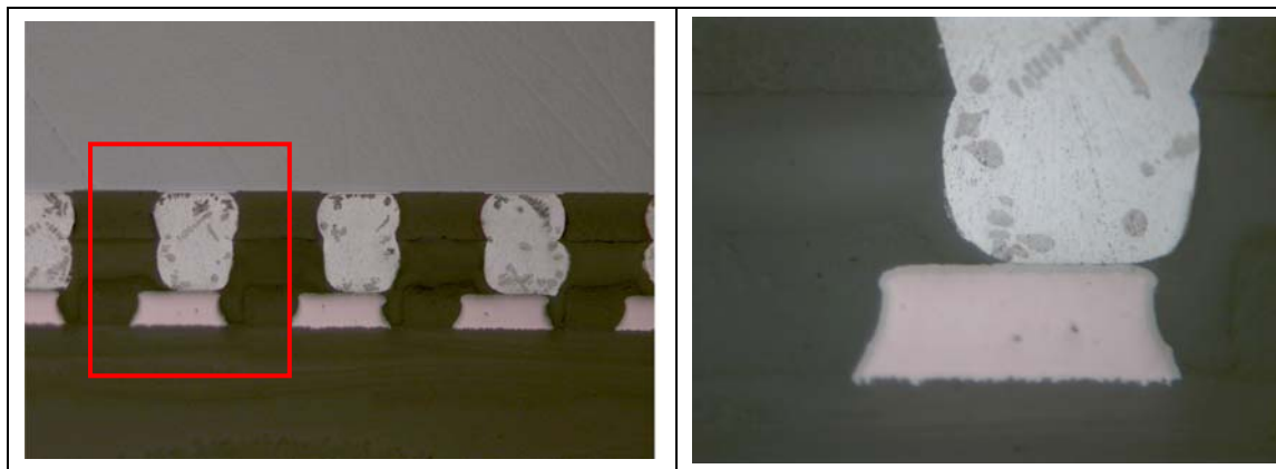
Figure 4.20 Non-wetting solder joint of double bump flip chip
