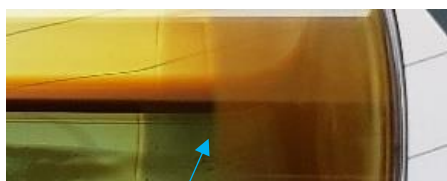
Figure 6.1: Precipitation on sides of bottle after ~36 hrs
