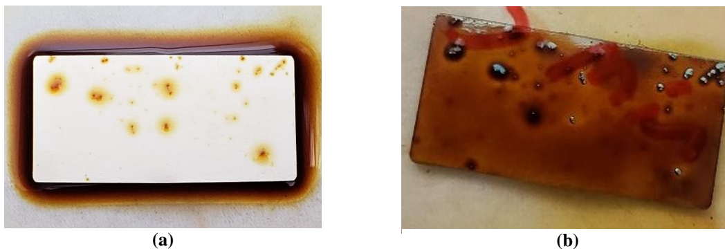
Figure 6.13: 1.3 wt% dodecane after 24 hrs (a) and 38 days (b)
