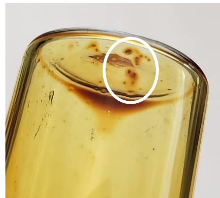
Figure 2.10: Proprietary solvent colloid 'separation' (inside white circle)
