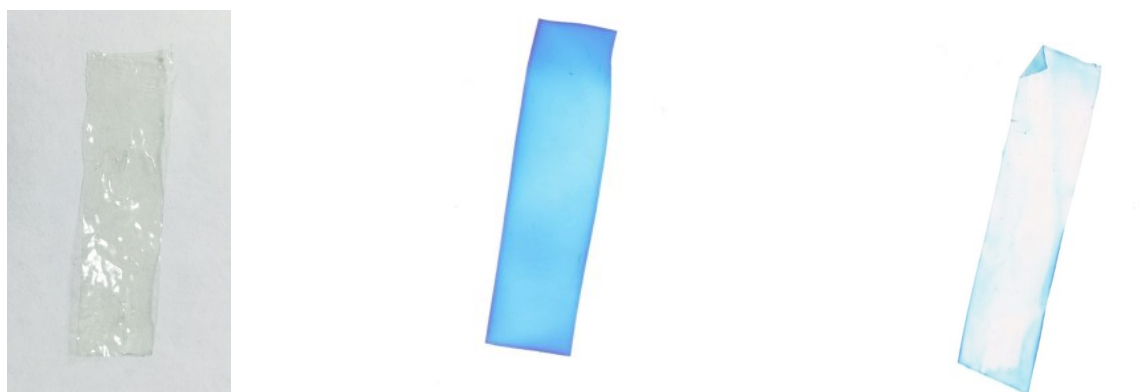
Figure 3.2: a) A washed SPEEK/PVA film b) Th-doped SPEEK/PVA film c) After 25 min of illumination of Th-doped film (30 wt% SPEEK and 70 wt% PVA). Film dimensions; 3 \text{ cm} \times 0.8 \text{ cm} \times 0.0075 \text{ cm} . SPEEK from Solvay precursor. I_0 = 10 \mu\text{M/s} and T = 25 \text{ }^\circ\text{C} .
