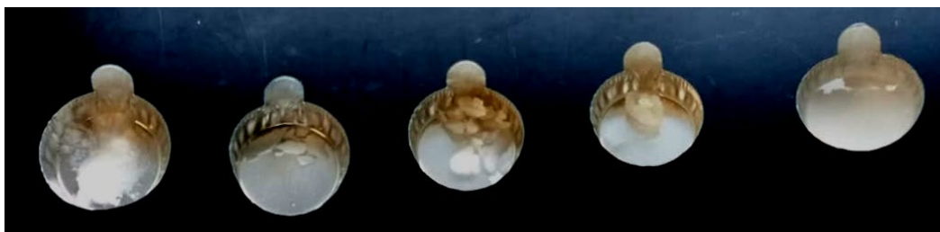
Figure 3.5.. Aluminum pans with the materials used for this work, from left to right: CD, PCD, CNF-PCD, CNF-CD, and CNF suspensions
