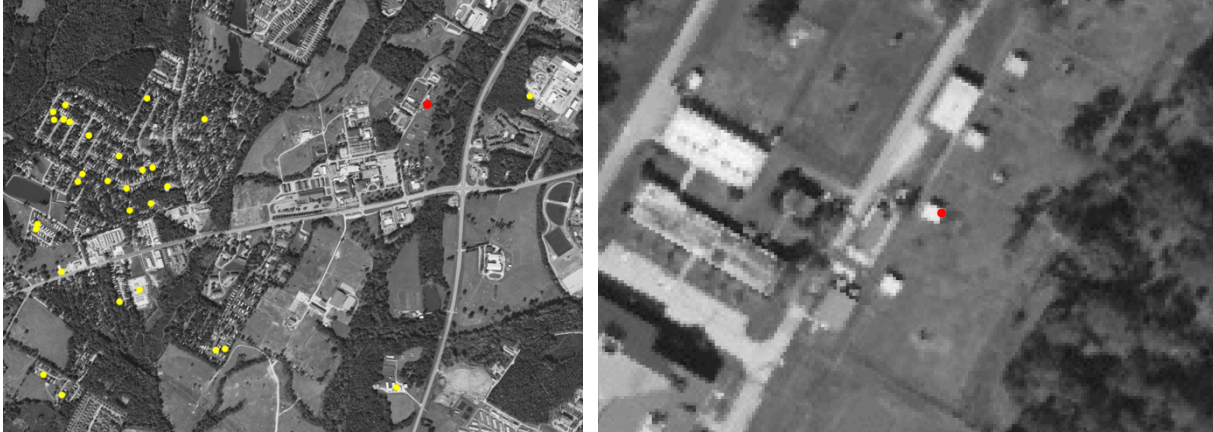
Figure 2.18: (Left) Corners detected in simulated sensed image from Google satellite maps with Shi Tomasi corner detection. Selected point for analysis is indicated by a red dot. (Right) Corner in a zoomed-in view of sensed image
