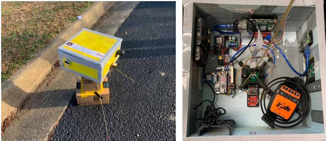
Figure A.3: (Left) Exterior of polystyrene payload container with quarter wave monopole antenna. (Right) Interior of payload box showing electronics.
