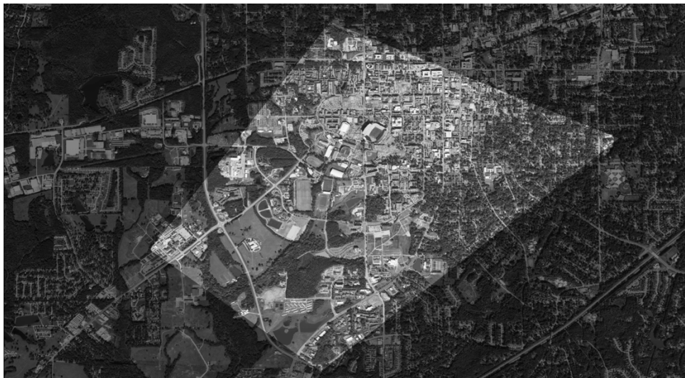
Figure 4.5: Correspondence between simulated sensed image and reference map with homography. Lighter shaded section is sensed image and darker shaded background is reference map.
