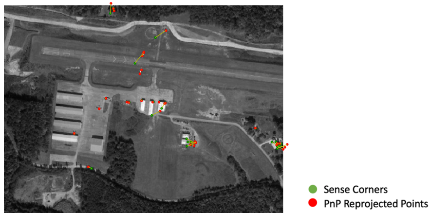
Figure 2.17: Reprojected sensed image points on Google satellite imagery reference map. The corresponding matches are indicated by yellow lines.
