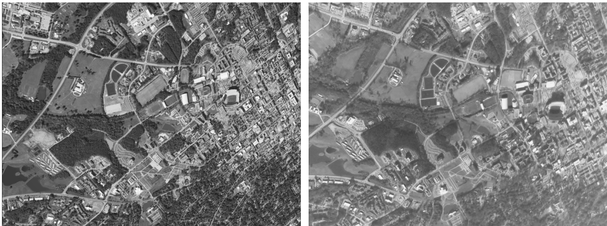
Figure 4.4: (Left) Simulated image with Google reference imagery (Right) Aerial image captured from High Altitude Balloon
