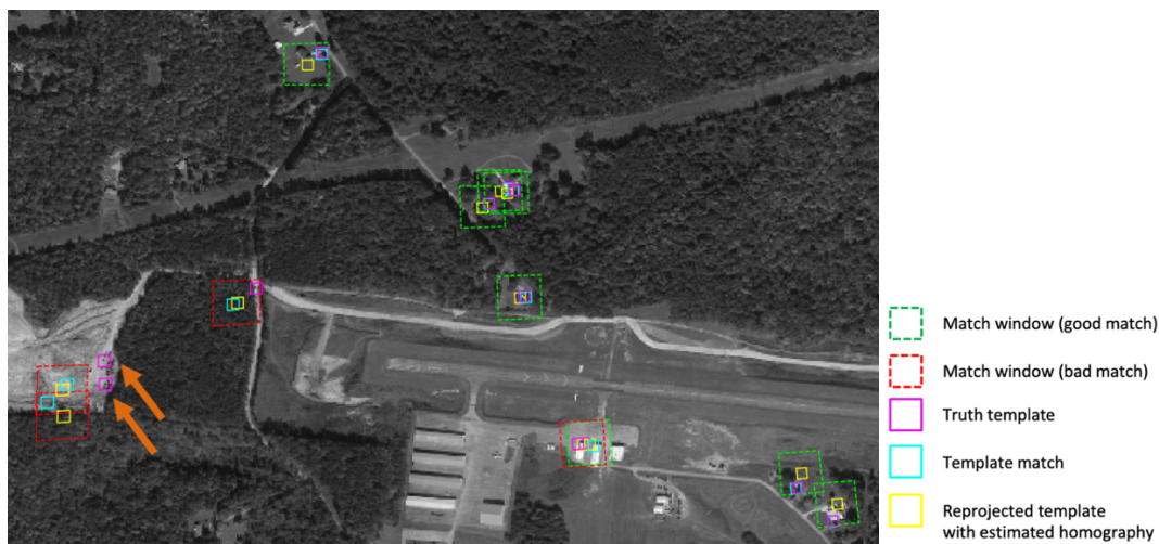
Figure 2.25: Matches with a sensed Google Satellite to reference Google Satellite image with rotation error of 3 degrees in pitch, roll, and yaw. Matches where truth template is outside of window are indicated with orange arrows.
