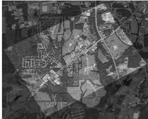
Figure 2.19: (Lighter foreground) Google satellite maps simulated sensed image overlapped with (Darker background) Bing aerial maps reference image with homography
