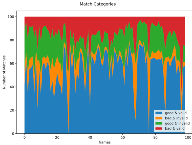
Figure 6.10: Stacked plot of matched category distribution for each frame. A good match is one that is within 50 pixels of the truth. A match is valid if its correlation passes the height and width criteria.
