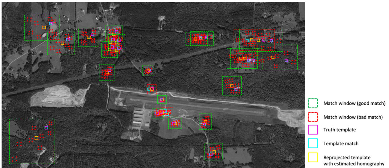
Figure 2.28: Google sensed to Google reference image with 3 degrees error in pitch, roll, and yaw with dynamic window sizing implemented.
