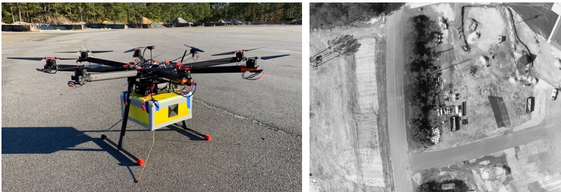
Figure 5.1: (Left) Tarot octocopter outfitted with data collection system. (Right) Example image captured by down-look camera.
